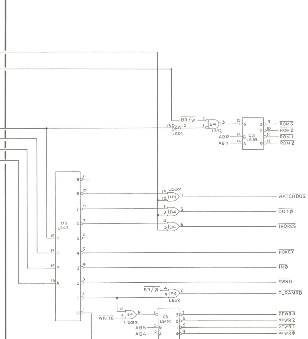
The MPU address decoding circuitry turns on or enables the appropriate game circuitry (i.e., RAM, ROM, latches, etc.) at the correct time, so that information can be transferred back and forth between the game circuitry and the MPU.
