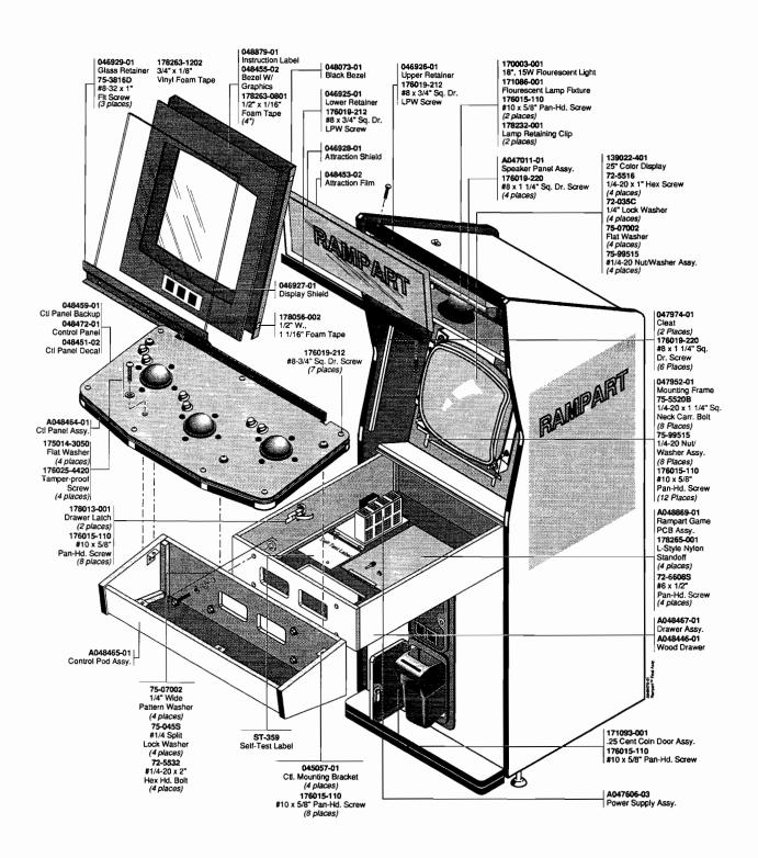
Figure 4-1 Cabinet-Mounted Assemblies A048470-01 B
