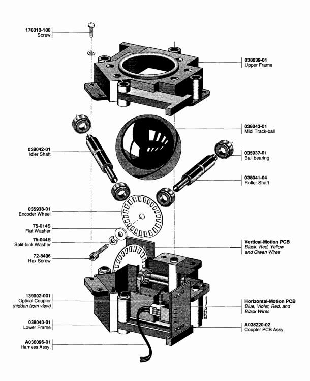
Figure 4-3 Midi Trak-Ball Assembly A038038-01 F
