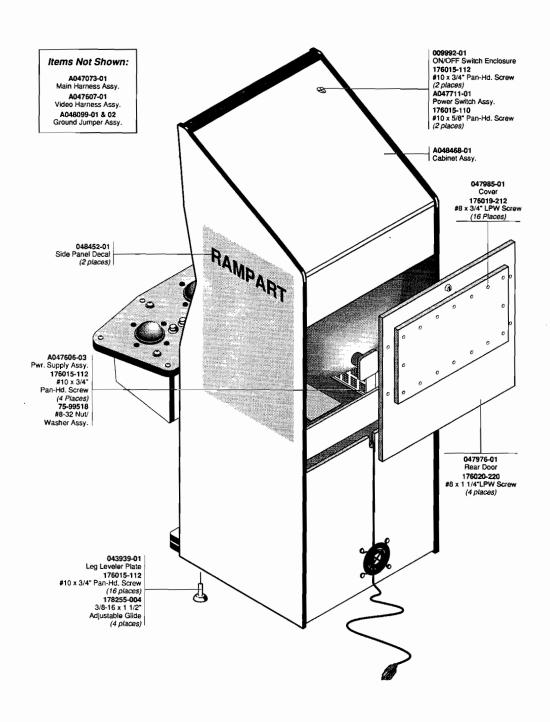
Figure 4-1 Cabinet-Mounted Assemblies A048470-01 B
