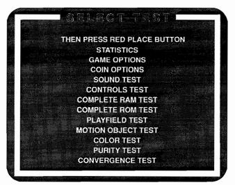
Figure 2-1 Self-Test Menu Screen
