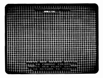
Figure 2-12 Convergence Test Screen
