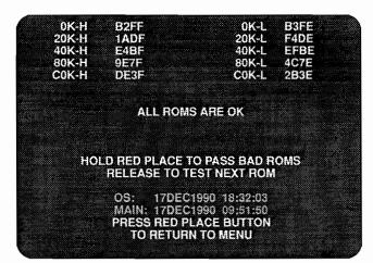
Figure 2-8 Complete ROM Test Screen
