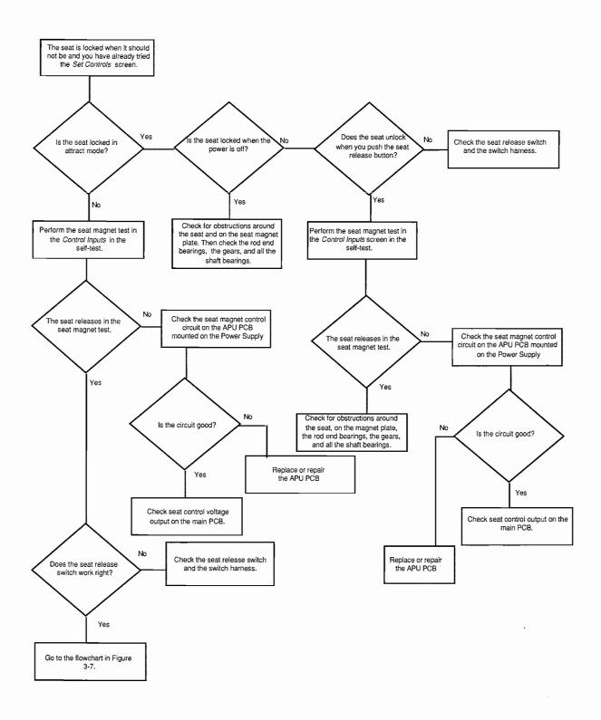
Figure 3-14 Seat is Locked When It Should Not Be And You Have Already Tried the *Set Controls* Screens
