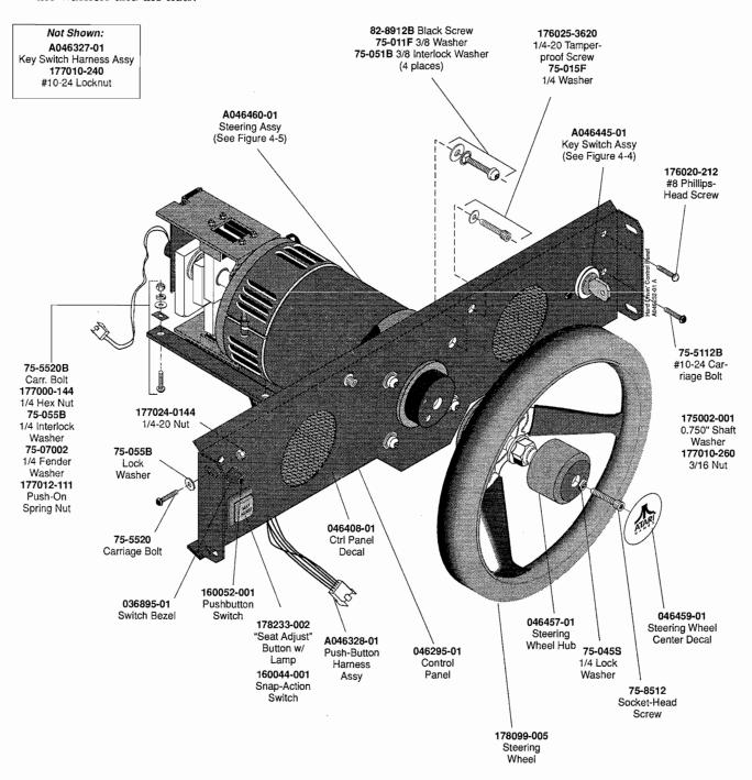
Figure 3-1 Removing and Installing the Dashboard
