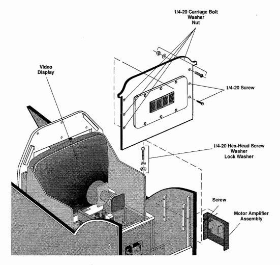
Figure 3-16 Removing the Video Display
