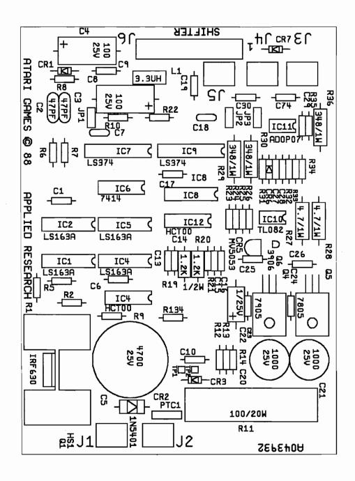
Figure 4-13 Shifter PCB Assembly A043932-01 C
