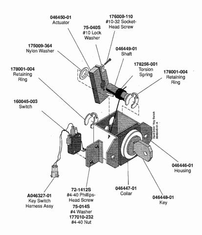
Figure 3-6 Maintaining the Key Switch Assembly
