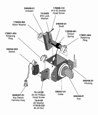
Figure 4-4 Key Switch Assembly A046445-01 B
