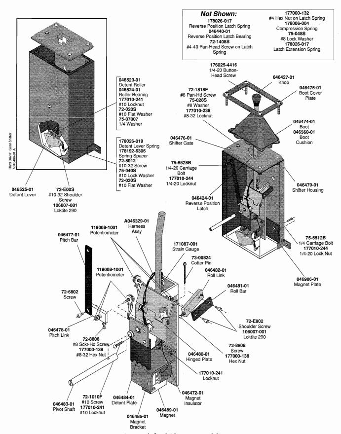
Figure 4-6 Shifter Assembly A046486-01 A
