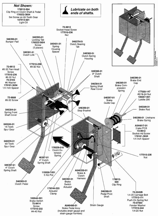
Figure 3-8 Maintaining the Clutch and Brake Assembly
