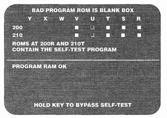
Figure 2-1 Program ROM and RAM Test
