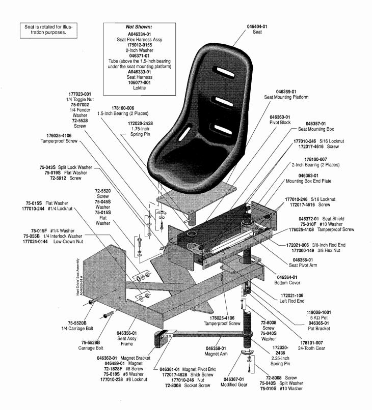
Figure 3-15 Maintaining the Seat Assembly
