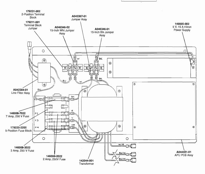
Figure 4-10 Power Supply Assembly A046345-01 A
