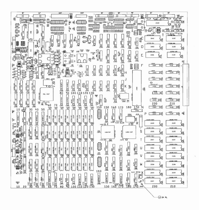
Figure 4-11 Hard Drivin' Main PCB Assembly A044425-01 C
