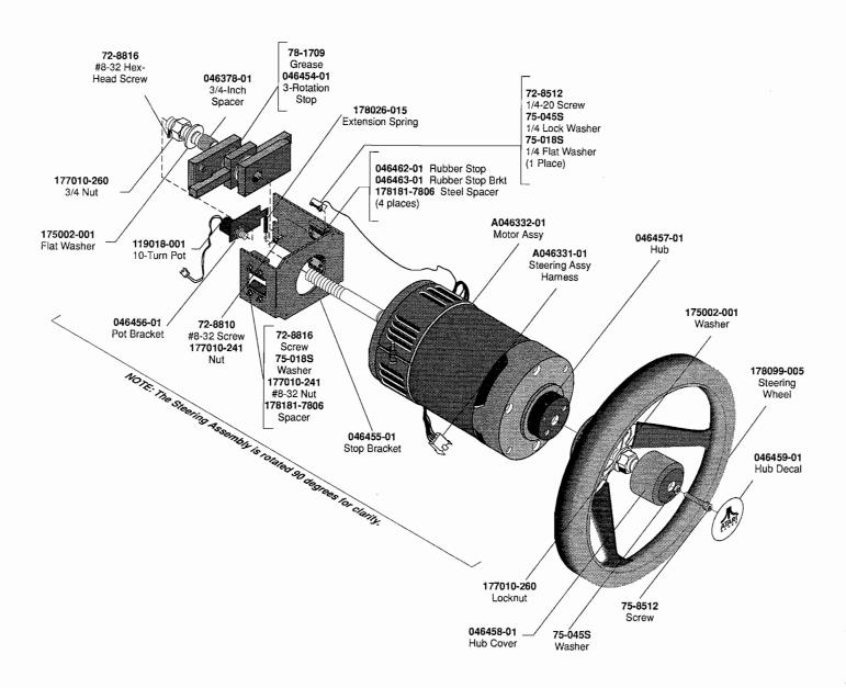
Figure 4-5 Steering Assembly A046460-01 A
