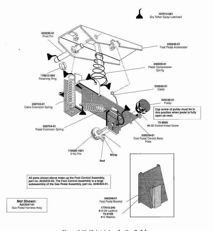
Figure 3-10 Maintaining the Gas Pedal
