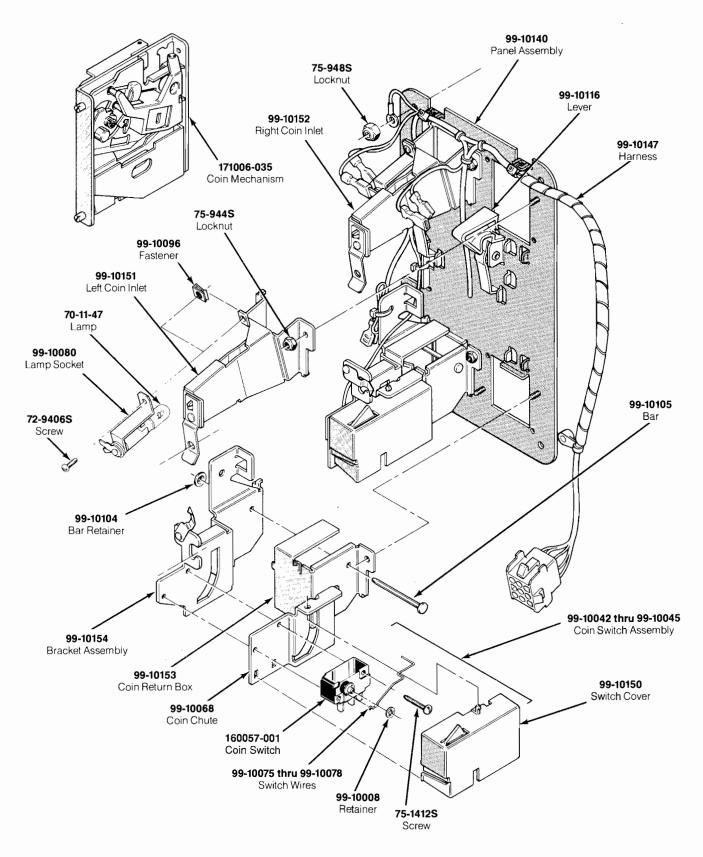
Figure 4-9 Coin Acceptors, Inc. Coin Door Assembly 171027-001 A
