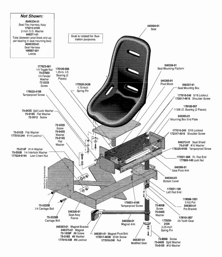
Figure 4-2 Seat Assembly A046355-01 A
