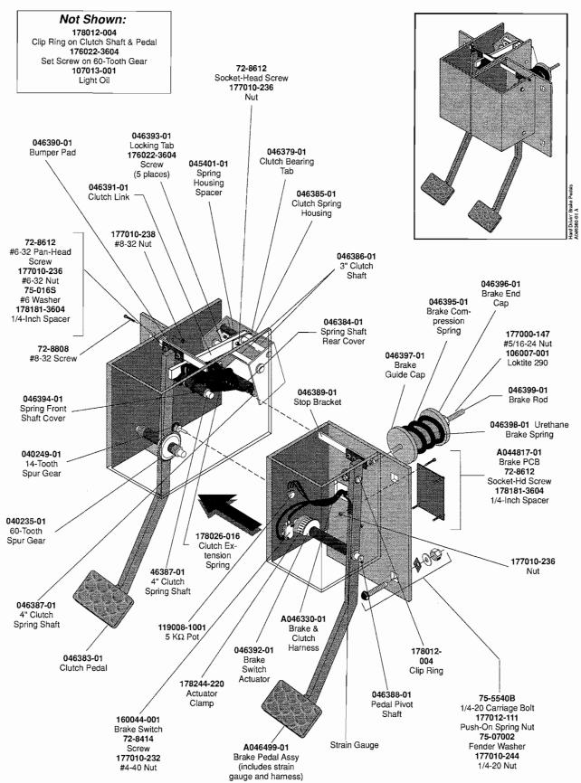
Figure 4-7 Clutch And Brake Pedal Assembly A046380-01 A
