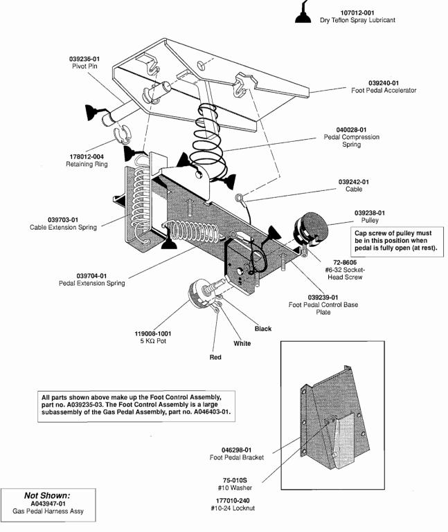
Figure 4-8 Gas Pedal Assembly A046403-01 E
