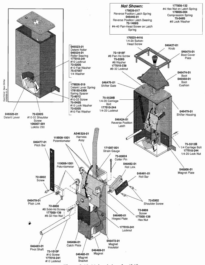
Figure 3-12 Maintaining the Shifter
