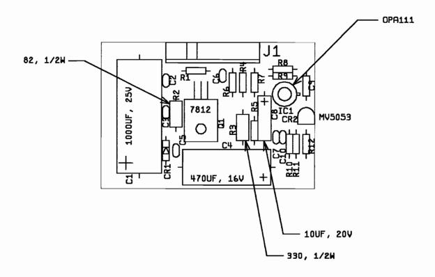
Figure 4-14 Brake PCB Assembly A044817-01 B
