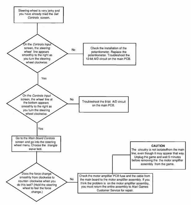
Figure 3-4 Steering Wheel Is Very Jerky and You Have Tried the Set Controls Screens
