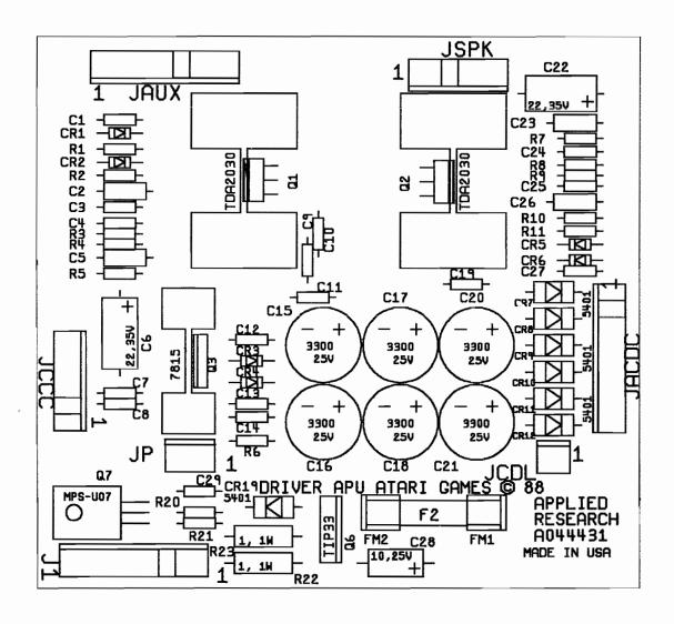
Figure 4-12 APU PCB Assembly A044431-01 B
