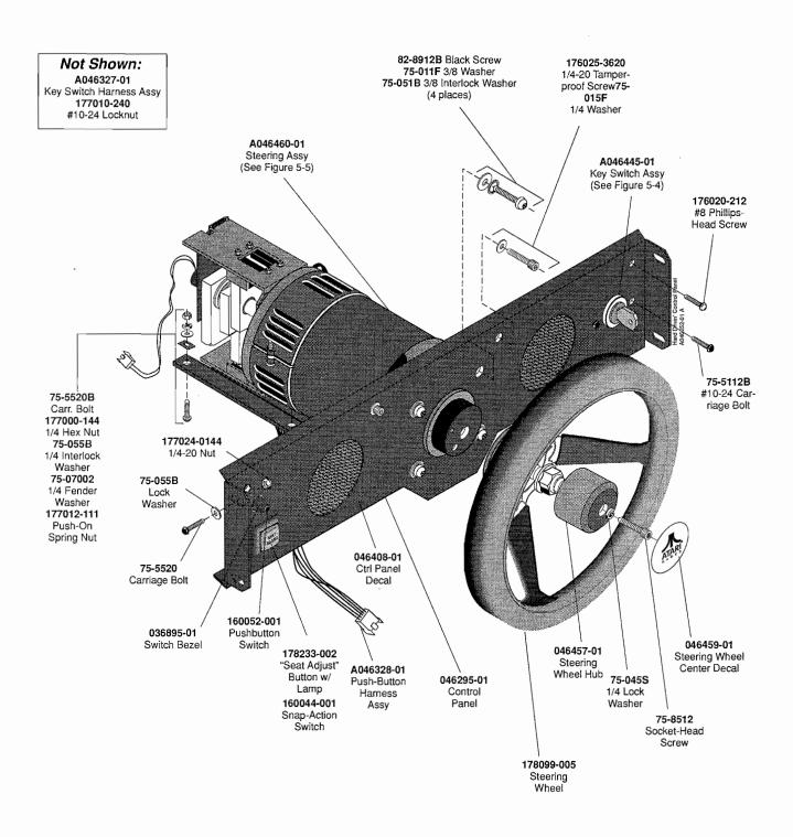
Figure 4-3 Dashboard Assembly A046252-01 A
