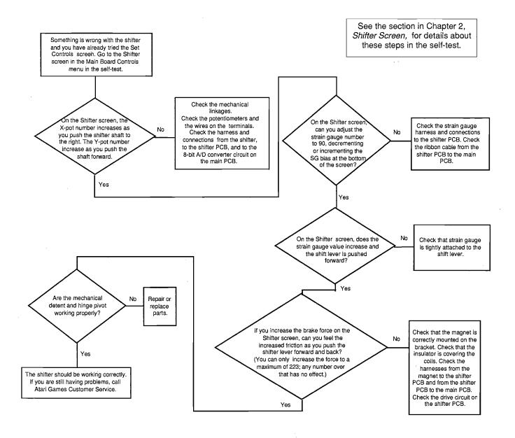
Figure 3-11 Shifter Is Not Working or Working Erratically And You Have Already Tried the *Set Controls* Screens
