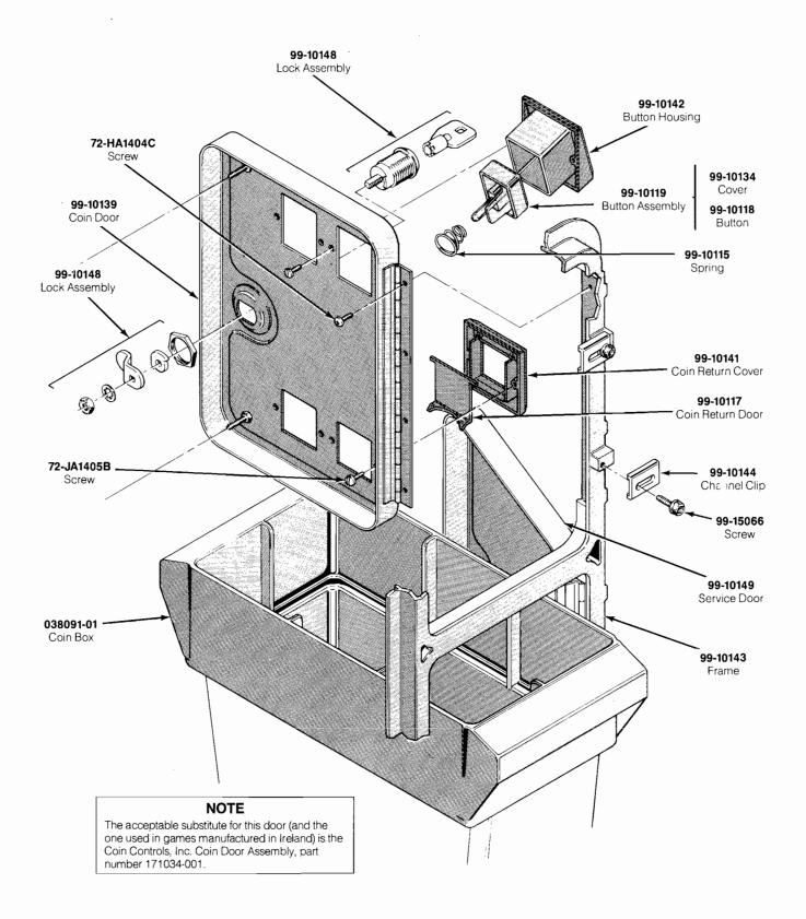
Figure 4-9 Coin Acceptors, Inc. Coin Door Assembly, Continued 171027-001 A
