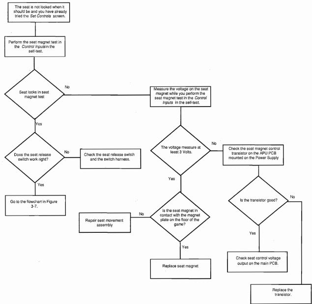
Figure 3-13 Seat is Not Locked When It Should Be And You Have Already Tried the Set Controls Screens
