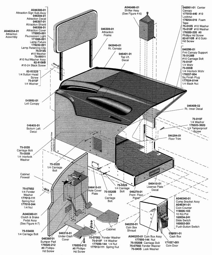
Figure 4-1 Cabinet-Mounted Assemblies, Front View A046250-01 B
