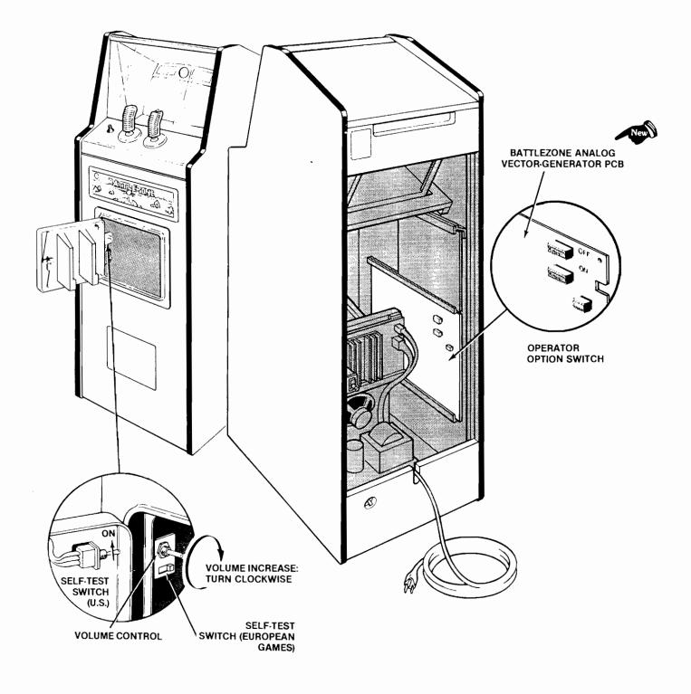
Figure 5 Location of Self-Test Switch, Volume Control and Option Switches
