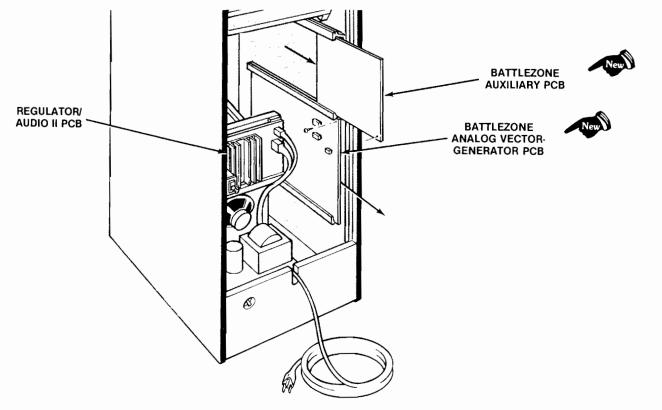
Figure 13 Printed-Circuit Board Replacement
