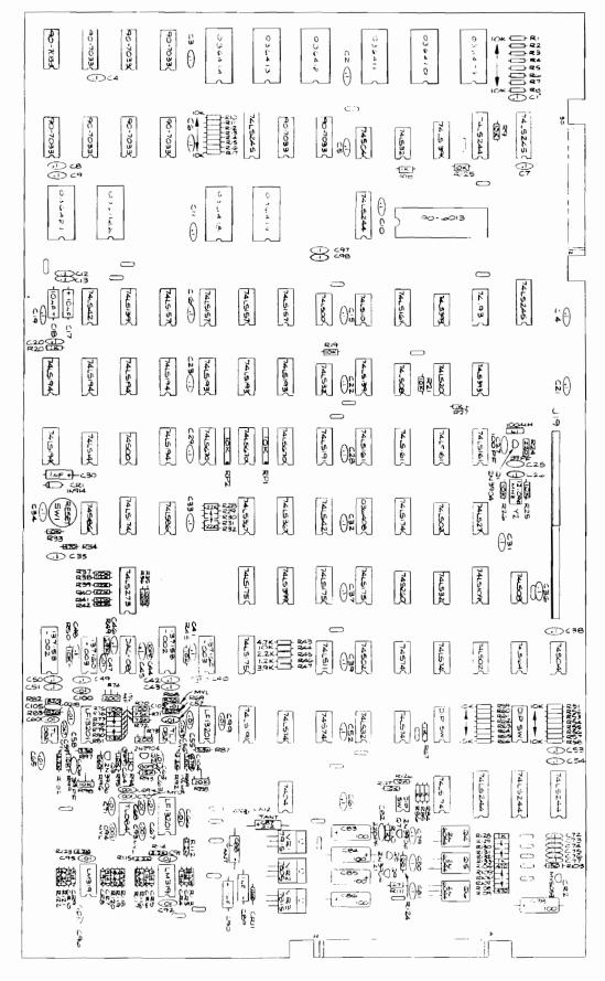
Figure 23 Battlezone<sup>™</sup> Analog Vector-Generator PCB Assembly A036424-02 A
