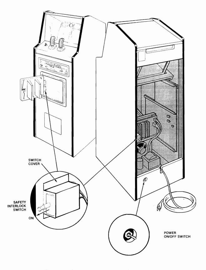
Figure 4 Interlock and Power On/Off Switches
