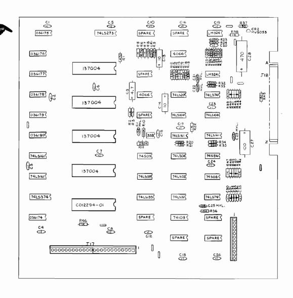
Figure 22 Battlezone™ Auxiliary PCB Assembly A035678-01 B
