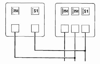
This pattern is important for you to know, so you can correctly set the "multipliers" for each mech. The multipliers determine how much each mechanism will be worth to the game's logic.
