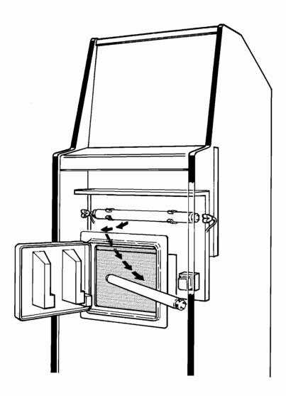
Figure 14 Fluorescent Tube Replacement
