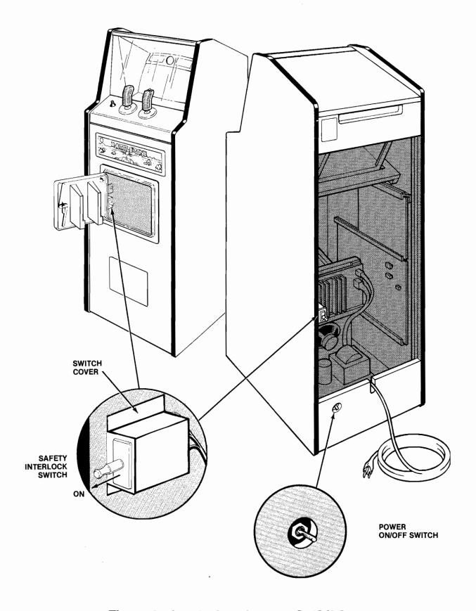
Figure 4 Interlock and Power On/Off Switches
