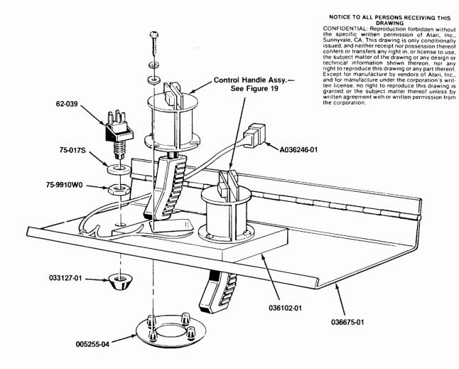
Figure 18 Control Panel Assembly A036656-01 A
