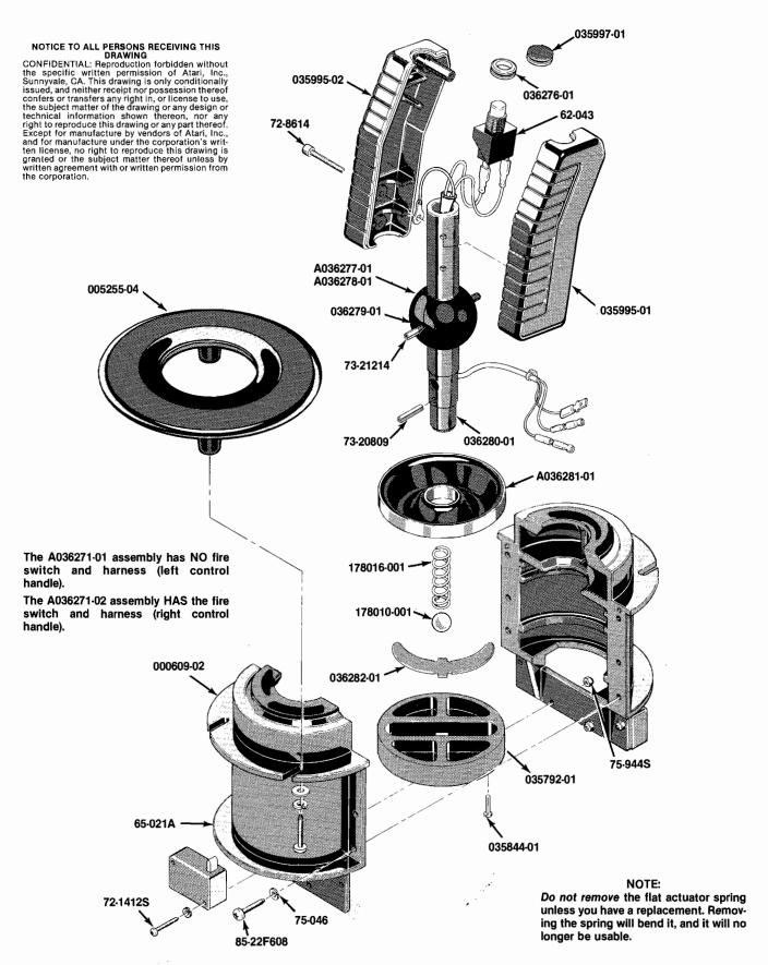
Figure 19 Control Handle Assembly A036271-01 and -02 B
