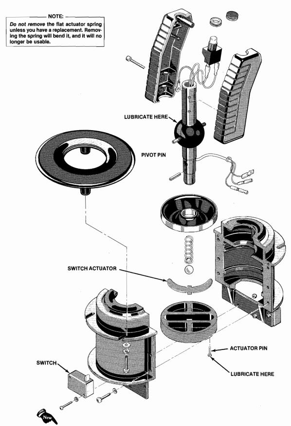
Figure 11 Control Handle Maintenance and Repair
