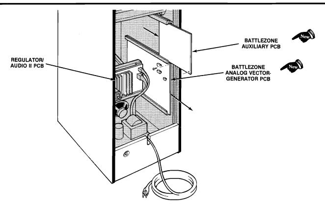
Figure 13 Printed-Circuit Board Replacement
