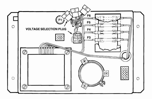
Figure 3 Line Voltage Selection
