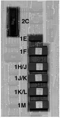
You'll be replacing the PROMs (on the left, 7H-7L); removing the EPROMs (on the right, 1F-1M); removing the NOVRAM at 1E; removing the CPU at 2C; and placing the daughtercard in the socket at 2C, 1E and one pin at 1F.
