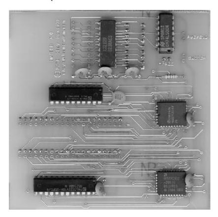
These instructions describe how to install the ESB 3.0/3.1 Daughtercard PCB into a Star Wars boardset with only requiring one cut on the Star Wars PCB (or an IC).
