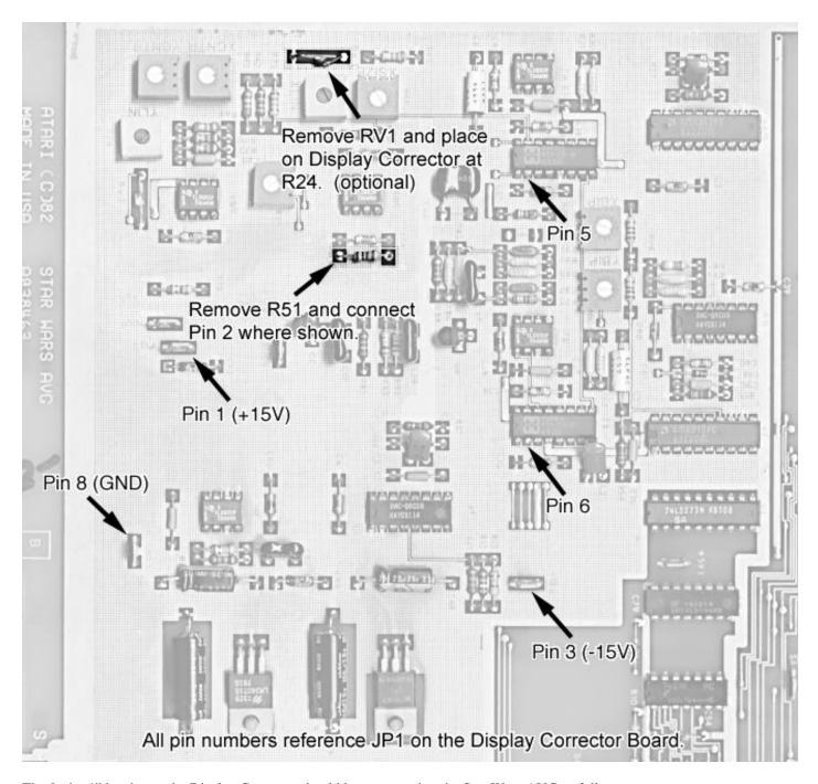
The 8-pin .1" header on the Display Corrector should be connected to the Star Wars AVG as follows:
