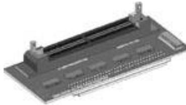
The 200-pin DIMM ADAPTER (p/n INN-8558-10) enables SIMCHECK II, or SIMCHECK II se, to test 200-pin FPM/EDO DIMM (Dual-Inline-Memory-Module) modules with a basic configuration of 144 bits used in the Sun Sparc Stations and other Sun Microsystem computers.
