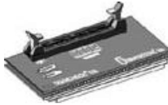
Our latest addition to the SIMCHECK II/IIse line provides a state-of-the-art solution for testing SDRAM/EDO/FPM 100-pin DIMM modules, which are typically used by Laser Printers. True 100MHz testing of your SDRAM is achieved through the Sync DIMMCHECK 100's patent pending 133MHz test engine.
