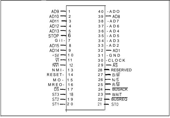
Figure 3-2. 28002 Pin Assignments
