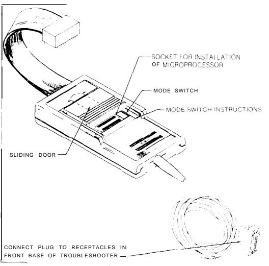
Figure 2-1. Location of Microprocessor Socket and Mode Switches
