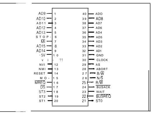
Figure 3.4. 28004 Pin Assignments
