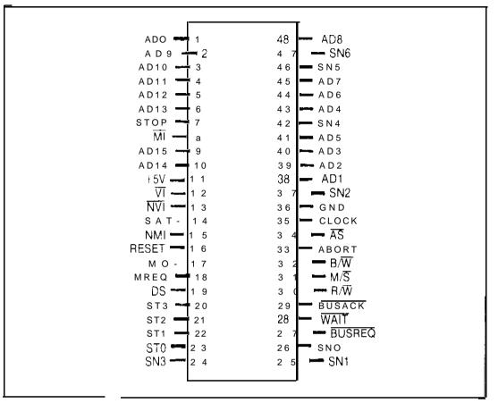
Figure 3-3. 28003 Pin Assignments
