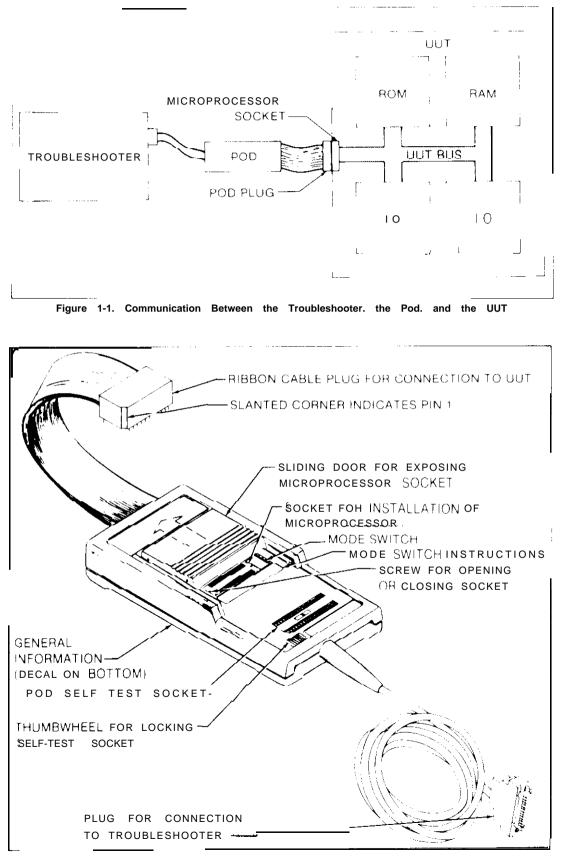
Figure 1-2, External Features of the Z8000 Interface Pod
