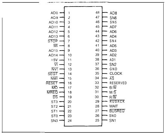
Figure 3-1. 28001 Pin Assignments
