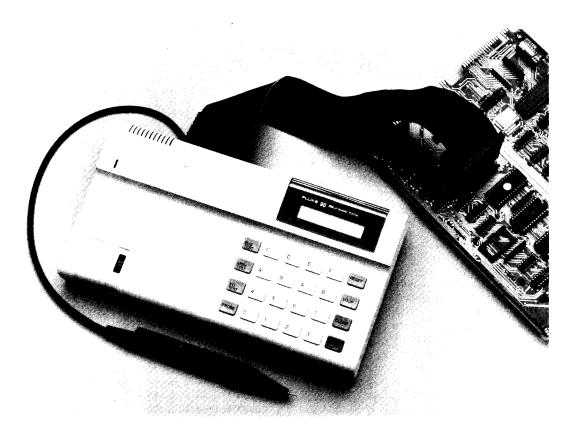
The tester contains several packaged test routines that automatically test bus lines, control lines, RAM (both dynamic and static), ROM and I/O functions. The built-in tests, invoked by pressing keys on the control panel, can be executed while the board-under-test is executing its own applications software.
