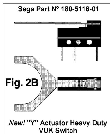
We have designed a **New! "Y" Actuator Heavy Duty VUK Switch** to be used in all of our new games and can replace all **Wire Loop Actuator VUK Switches** used on our previous games (used in various applications from **Last Action Hero** thru **Current Games**). The new switch uses the same heavy duty switch body we use on our **Ball Trough Switches** with a .030 thick flat metal actuator in a "Y" or "Fork" configuration (See Fig. 2A & 2B).
