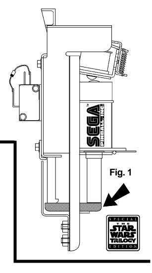
We have designed a **New!** "Y" **Actuator Heavy Duty VUK Switch** to be used in all of our new games and can replace all **Wire Loop Actuator VUK Switches** used on our previous games (used in various applications from **Last Action Hero** thru **Current Games**). The new switch uses the same heavy duty switch body we use on our **Ball Trough Switches** with a .030 thick flat metal actuator in a "Y" or "Fork" configuration (See Fig. 2A & 2B).
