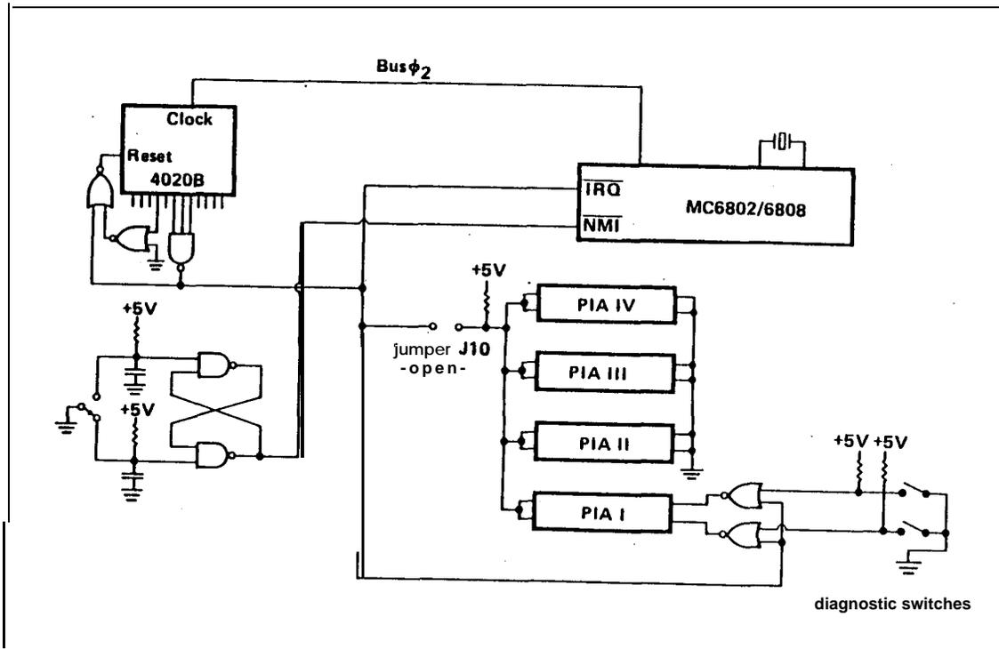
The  $\overline{\text{NMI}}$  input of the MC6802/MC6808 MPU is still used to start the diagnostic program. The interrupt generator circuit, though, has been replaced by an interrupt counter circuit. The 3.58 MHz crystal frequency is divided by 4 in the MC6802/MC6808 to about 900 kHz and is output as Bus $\phi$ 2. This signal is counted down by a 40208 CMOS counter. This chip has 14 counting stages with a clock input and reset input. Only 12 bits are output, though.
