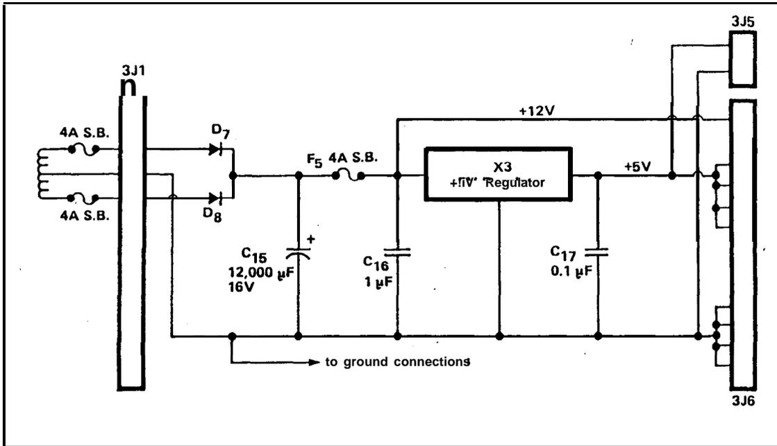
The logic supply fuse, F5, is rated at 4A and is a slow-blow type. In earlier games, this is the only fuse used in this supply. Capacitors C16 and C17 act as high frequency bypass capacitors and help prevent oscillation of the regulator. X3 may be replaced with an LM323K, LAS1405, or 78H05KC regulator.
