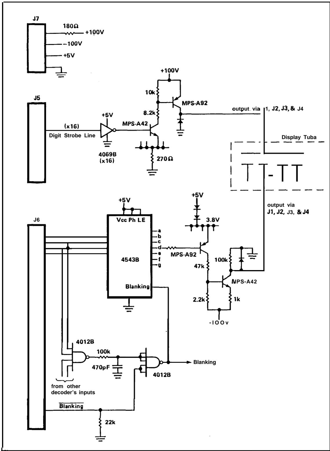
The 8.2k and 10k resistors are used to turn ON and turn OFF, respectively, the MPS-A92 driver. The clamp diode on the driver's collector protects the transistor from exposure to negative voltage spikes which may be applied to the anode due to the negative voltages on the segment cathodes in the display tube.
