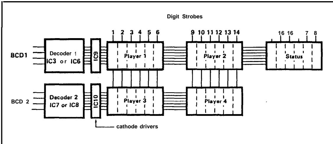
There are two types of master display boards used by Williams. The earlier type used IC drivers while the newer ones use discrete transistor drivers. The switch-over grew out of problems Williams had in obtaining sufficient quantities of their IC drivers. We will look at the earlier system first.
