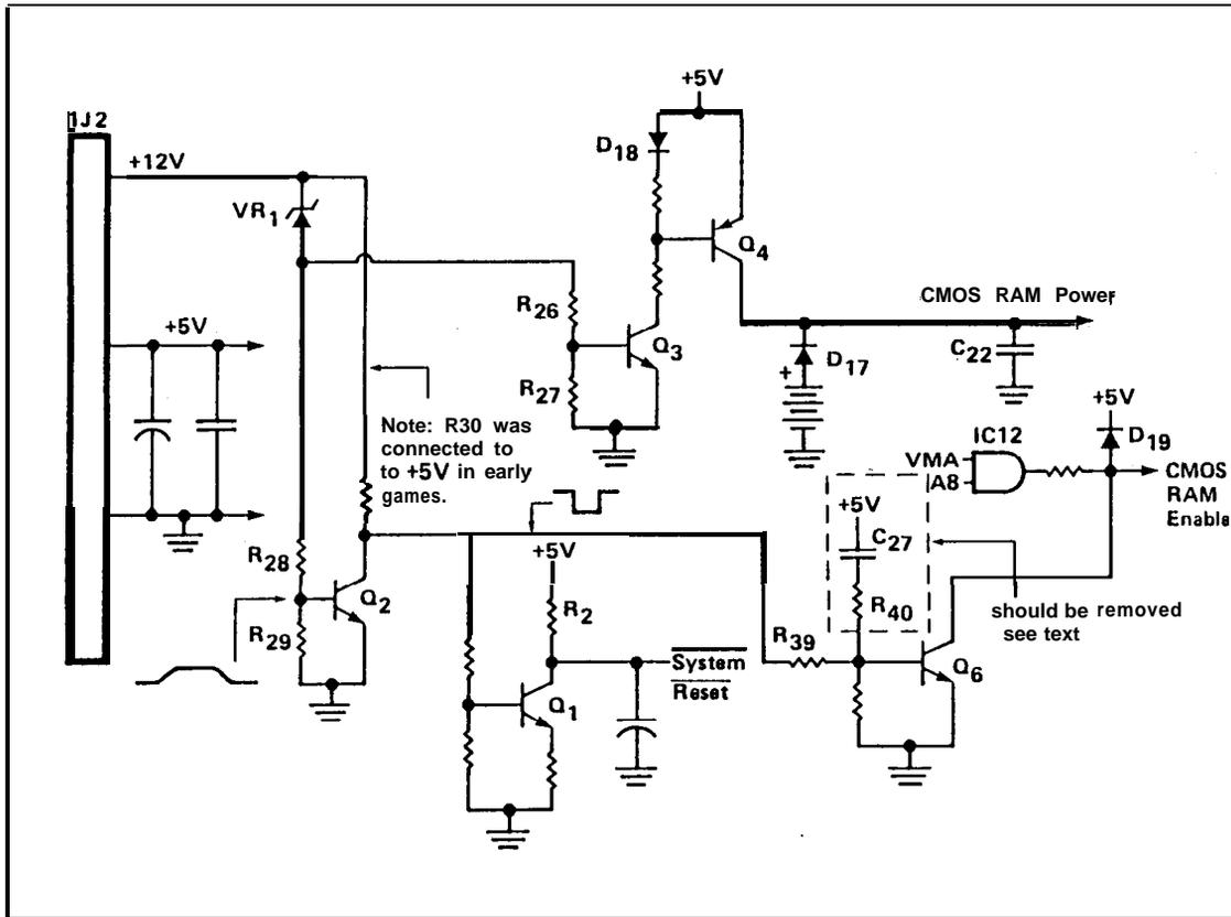
In some of the earlier games, C27 and R40 were used. If bookkeeping memory keeps being lost on those games, these two parts should be removed. R30 should be changed to 10k instead of 1k and be connected to the +12V supply.
