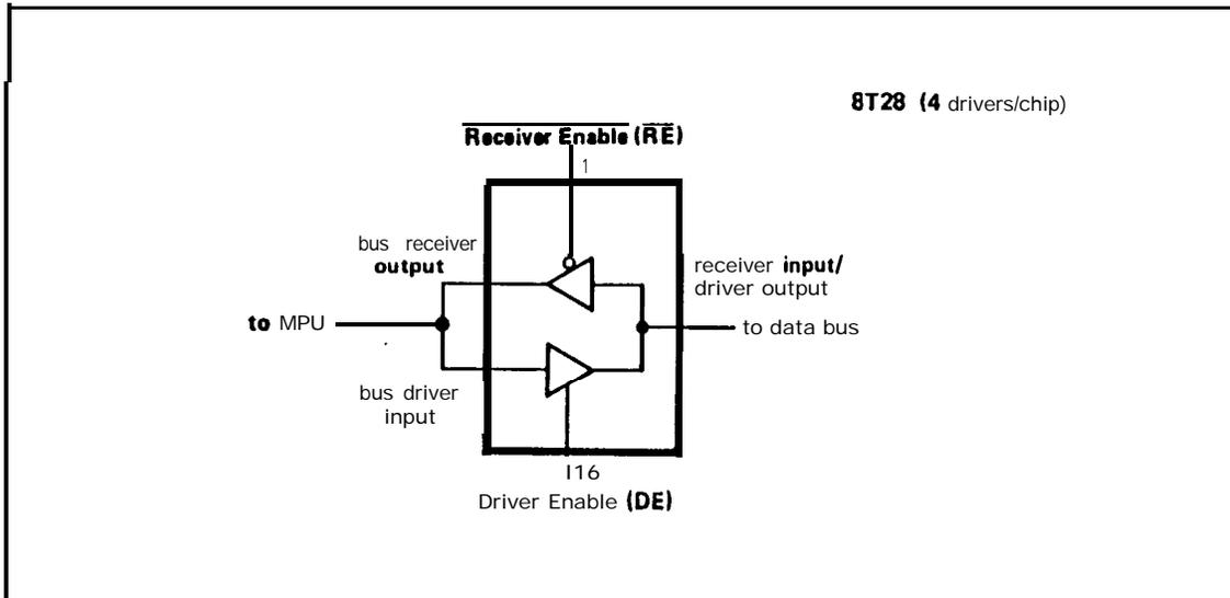
The bus drivers are required to drive all the parts on the bus on both the CPU board and driver board. Without them, at this high a clock frequency, the processor could not drive the voltage levels on the bus lines properly LOW and HIGH quickly enough.
