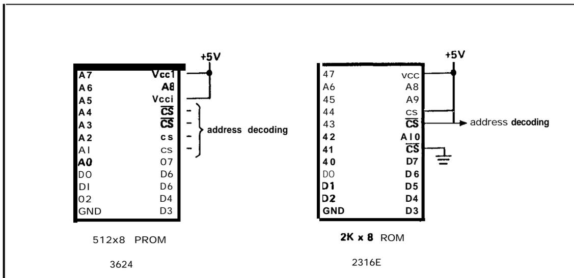
Program memory address decoding in the old CPU board is accomplished with three gates and an MSI decoder in two stages. First, part IC11, together with IC15, a BCD to decimal decoder, decode for the two utility ROMs and personality ROM/PROMs. Additional lines on the PROM chip selects further decode address lines A9 and A10. Note that only one output at a time is pulled LOW in the 7442, depending upon the BCD input code.
