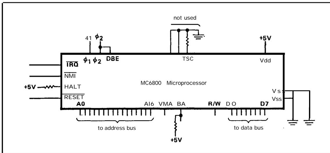
tion at a time. These inputs are controlled by IC11 pin 12. This is actually the signal  $\overline{VMA} \cdot \overline{BA} \cdot R/W \cdot \text{Bus} \cdot \phi 2 \cdot \text{RESET}$ . When this signal is LOW, data is transferred from the data bus to the MPU, and when HIGH, it is written from the MPU to external devices.
