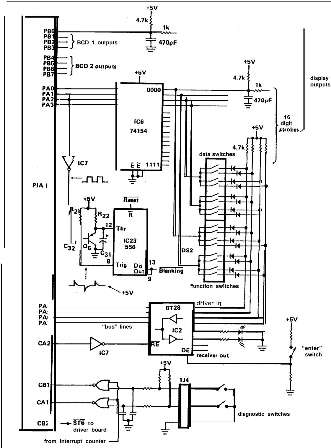
Column 1 of the switch matrix strobesc the front door and cabinet switches. Columns 2 through 8 are available for use on the playfield. The eight row returns are used in parallel in both the cabinet and playfield and the two sets are tied together physically at 2J3 on the upper right hand side of the driver board. Connector 2J2 above it carries the output strobes.
