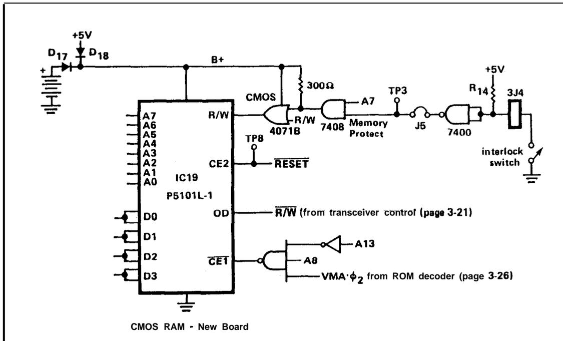
The interlock switch in the front door is opened whenever the front door is open. R14 pulls the 7400 NAND gate inputs HIGH, which causes one of the inputs of the 7408 AND gate to be pulled LOW. This causes the second input to the 40718 OR gate to be LOW and the CMOS RAM can then be written into.
