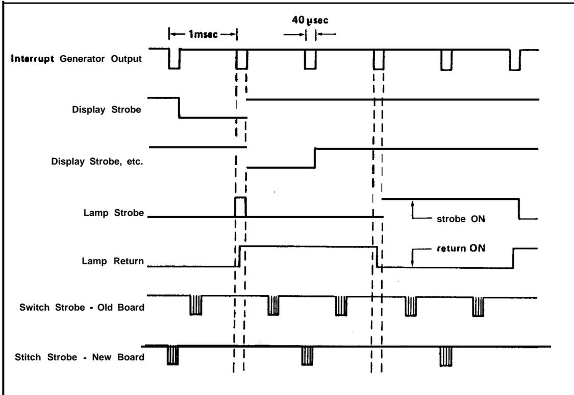
The interrupt generator runs at a frequency of about 1,100 Hz and the output signal has a period of about 900  $\mu$  sec.
