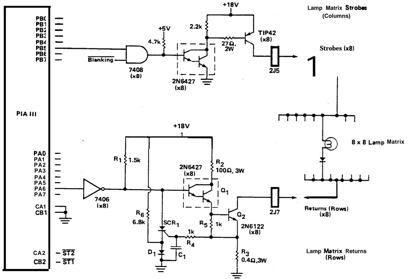
(column) lines to the playfield and insert board. Connector 2J7 connects the sixteen red 'urn (row) wires to the driver board.
