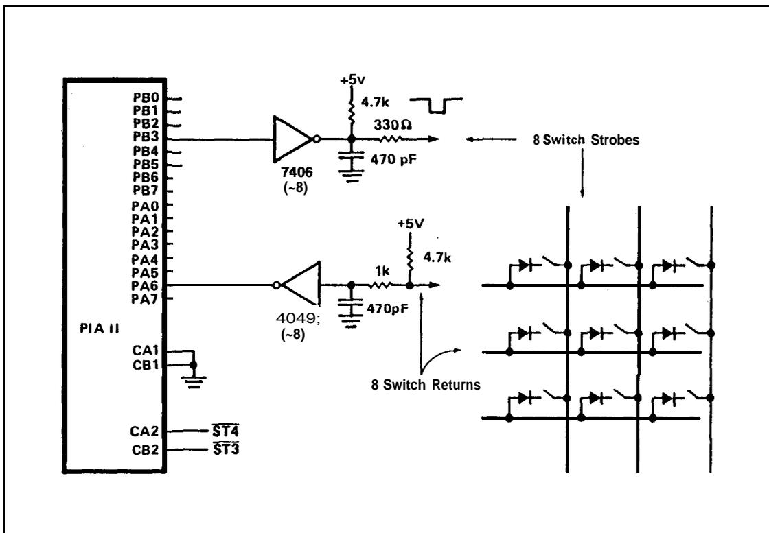
Both the strobe and return lines use 470pF capacitors, 4.7k pull-up resistors and 1 k series resistors. These deglitch the lines, provide static protection and provide momentary protection to both the strobes and returns in the event of accidental shorts on the playfield to lamps or solenoids.
