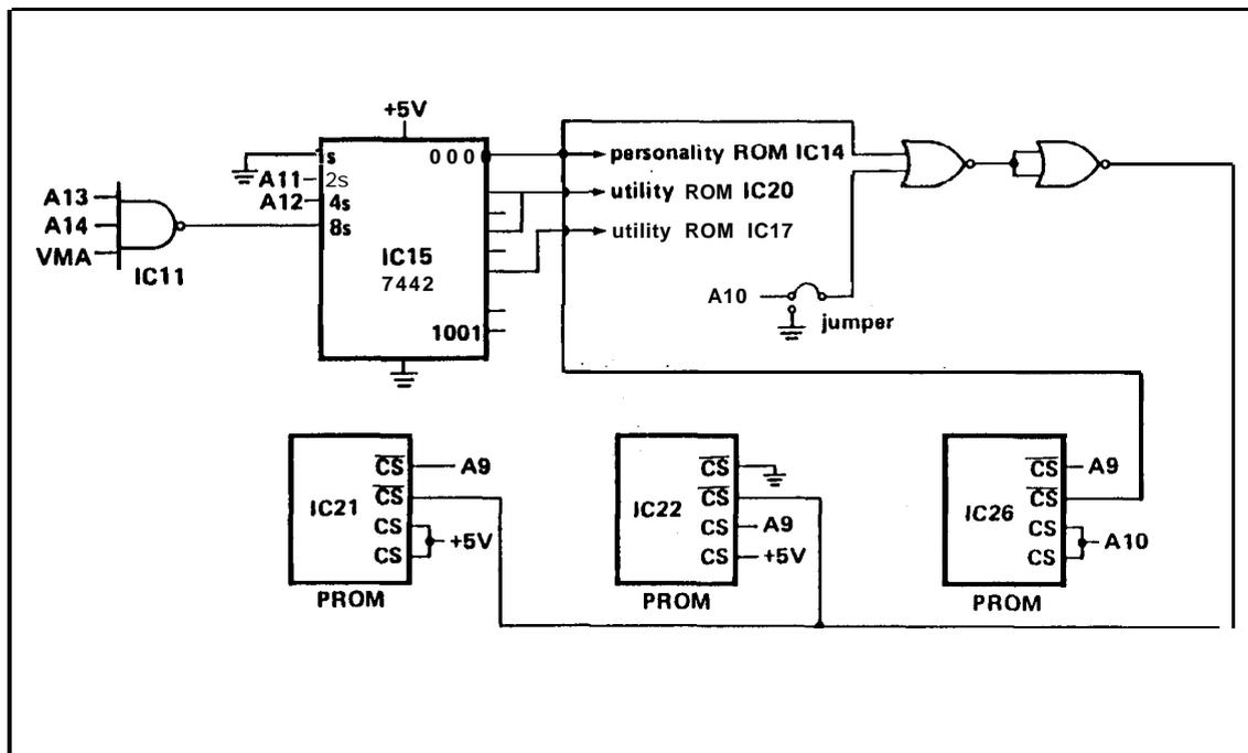
when program memory is to be accessed. The two utility ROMs at IC17 and IC20 are both enabled directly by the decoder. If a personality ROM at IC14 is used, it can be jumpered for one of two addresses (AI 1 HIGH or LOW). Addresses for personality PROMs are decoded further by the other half of the LS139.
