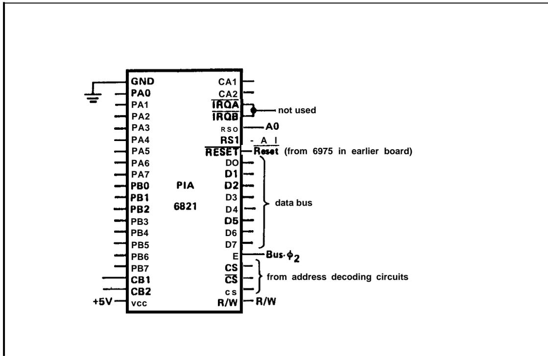
and  $\overline{\text{IRQB}}$  outputs do not connect to the MPU (see Interrupt Control of the system, pages 3-18 and 3-21).
