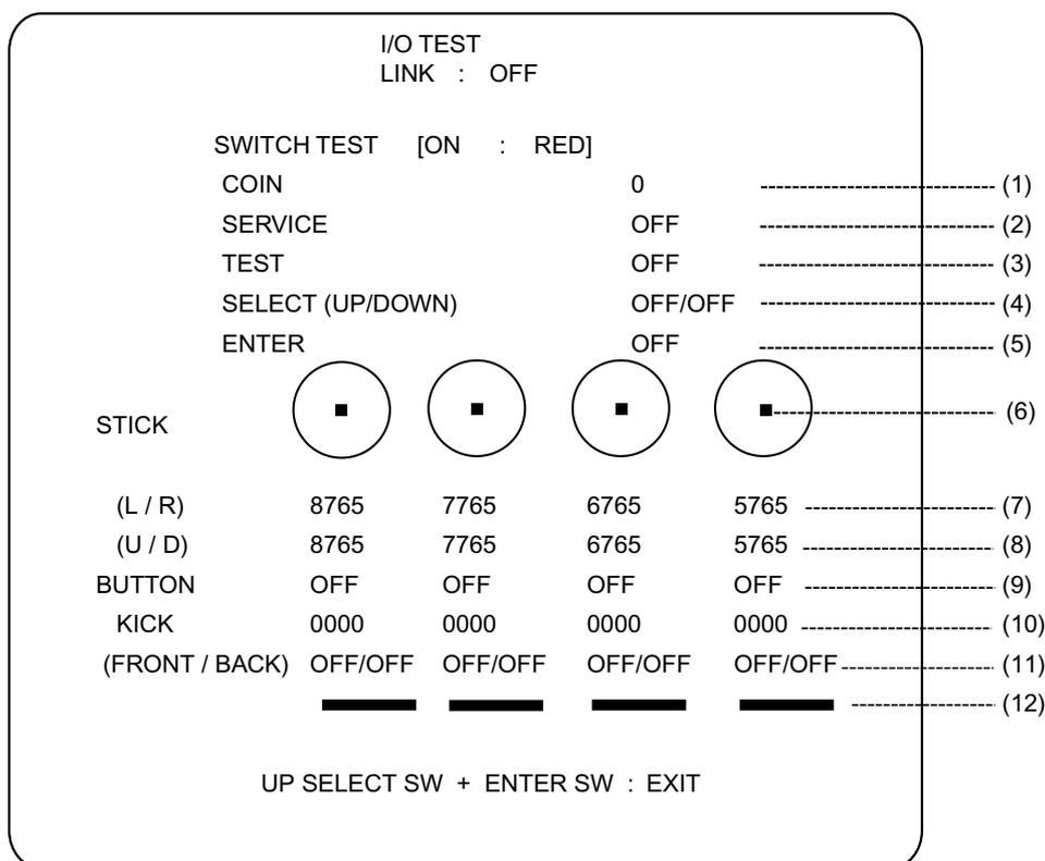
The SWITCH TEST screen displays the status of the switches. The display changes when any of the switches are operated. Press both Select Up switch and Enter Switch together to exit and return to the Menu.
