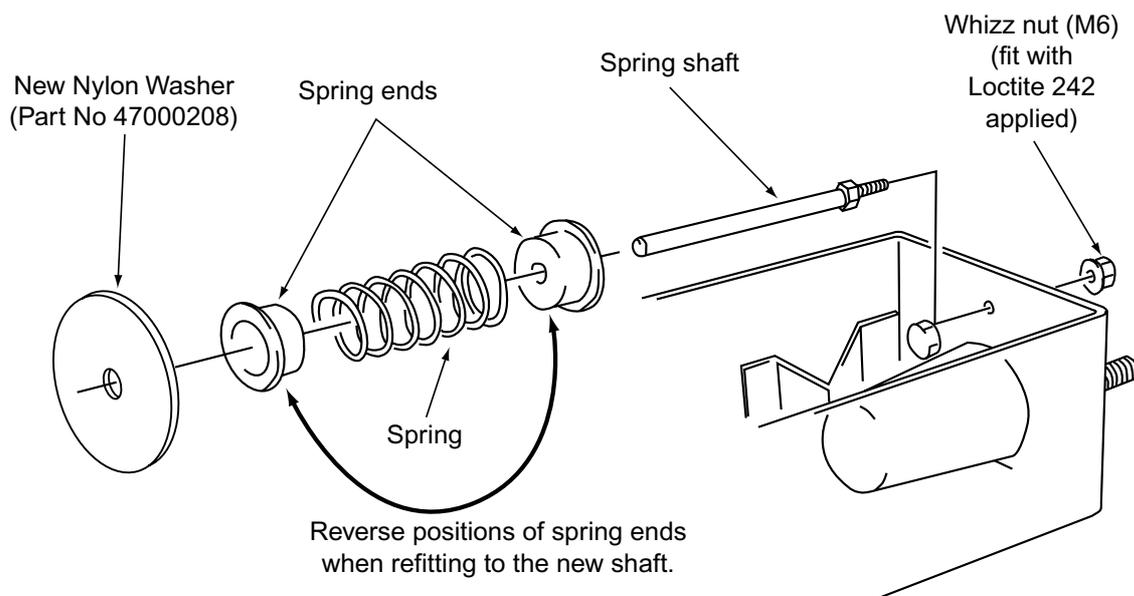
*Note: When tightening the Whizz nut ensure that the nut welded to the shaft is retained with a spanner to ensure that the Whizz nut is fully tightened. Failure to tighten the Whizz nut fully may allow the shaft to come loose during game play causing damage to the shaft.*
