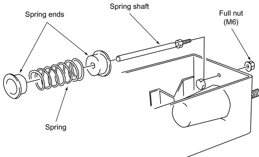
2. When reassembling the new Spring Shaft refit the spring ends in the opposite positions (front spring end refitted to the back and the back spring end refitted to the front).
