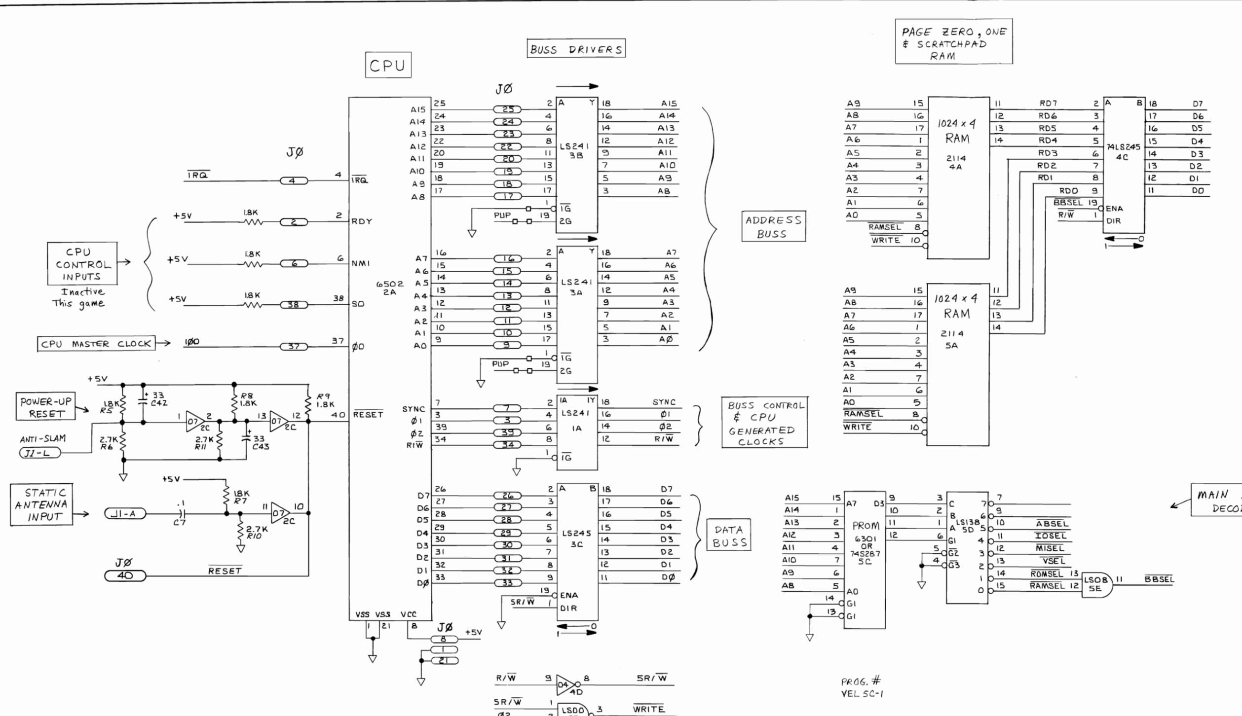
NOTE: Connector J0 used for test & analysis purposes only. Contains all CPU connections.
