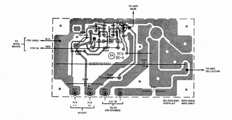
+5 Volt Supply Circuit Card Detail - Solder View
