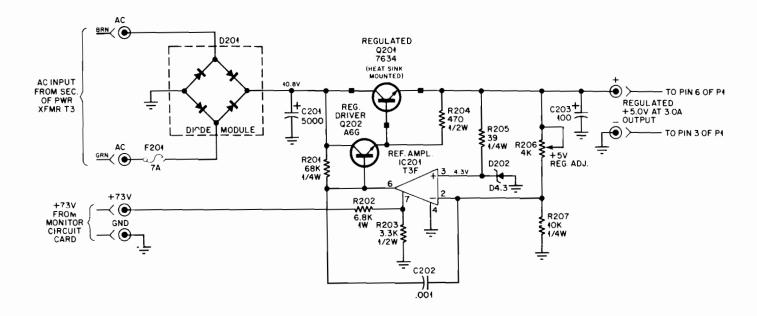
+5 Volt Supply - Diagram Schematic
