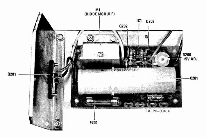
+5 Volt Circuit Card Detail - Component Location
