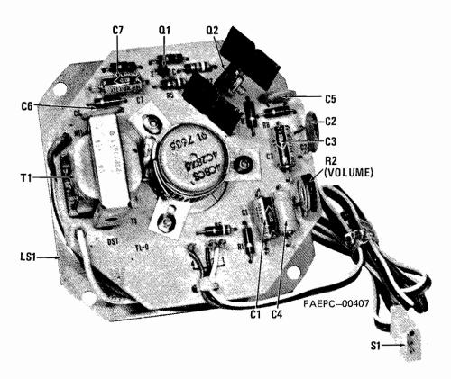
Audio Module - Circuit Card Detail - Component Location
