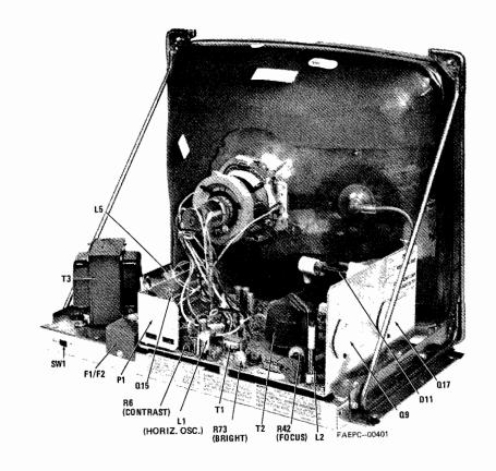
M5000-155, M7000-155, Chassis Rear View - Component Location
