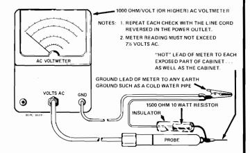
Voltmeter Hook-up for Safety Check
