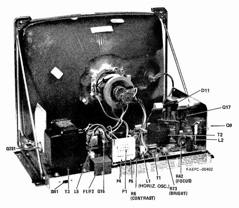
M5010-155, M7010-155, Chassis Rear View - Component Location
