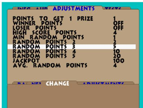
While ADJUSTMENTS is highlighted, the descending menu will show a subset of the system adjustments, since there are more than can fit on the screen at one time. If the adjustments have been automatically reset due to error since the last entry to service mode, that will also be noted. If an adjustment is shown in blue, it is disabled because of another adjustment. For instance, while PAYOUT
