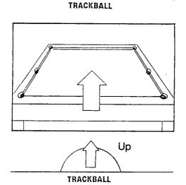
When the trackball is rolled forward the front of the table should move up.
