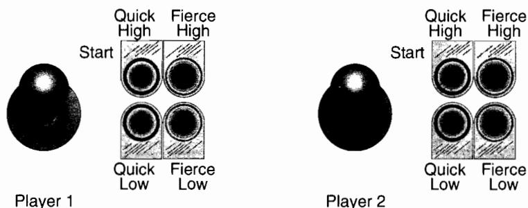
**Figure 1-2** Named Locations of Control Panel Assemblies
