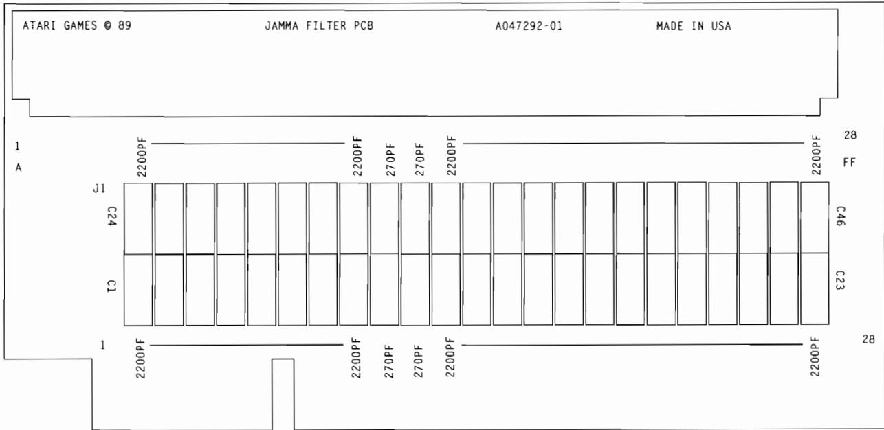
**Figure 4-5 JAMMA Filter PCB Assembly**
