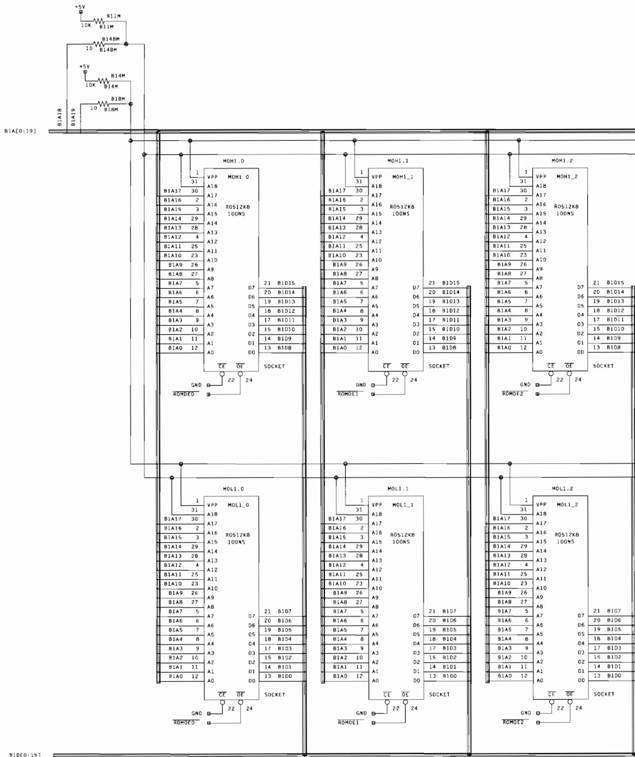
Figure 5-2 GT24M8 PCB Schematic Diagram
