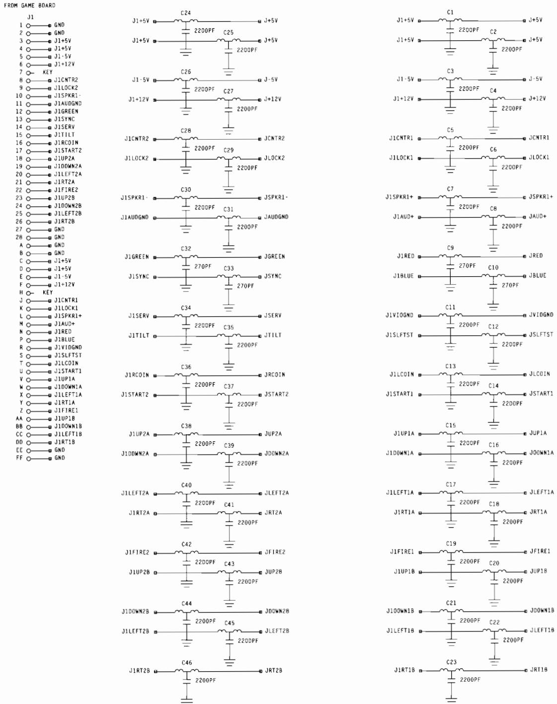
Figure 5-3 JAMMA Filter PCB Schematic Diagram
