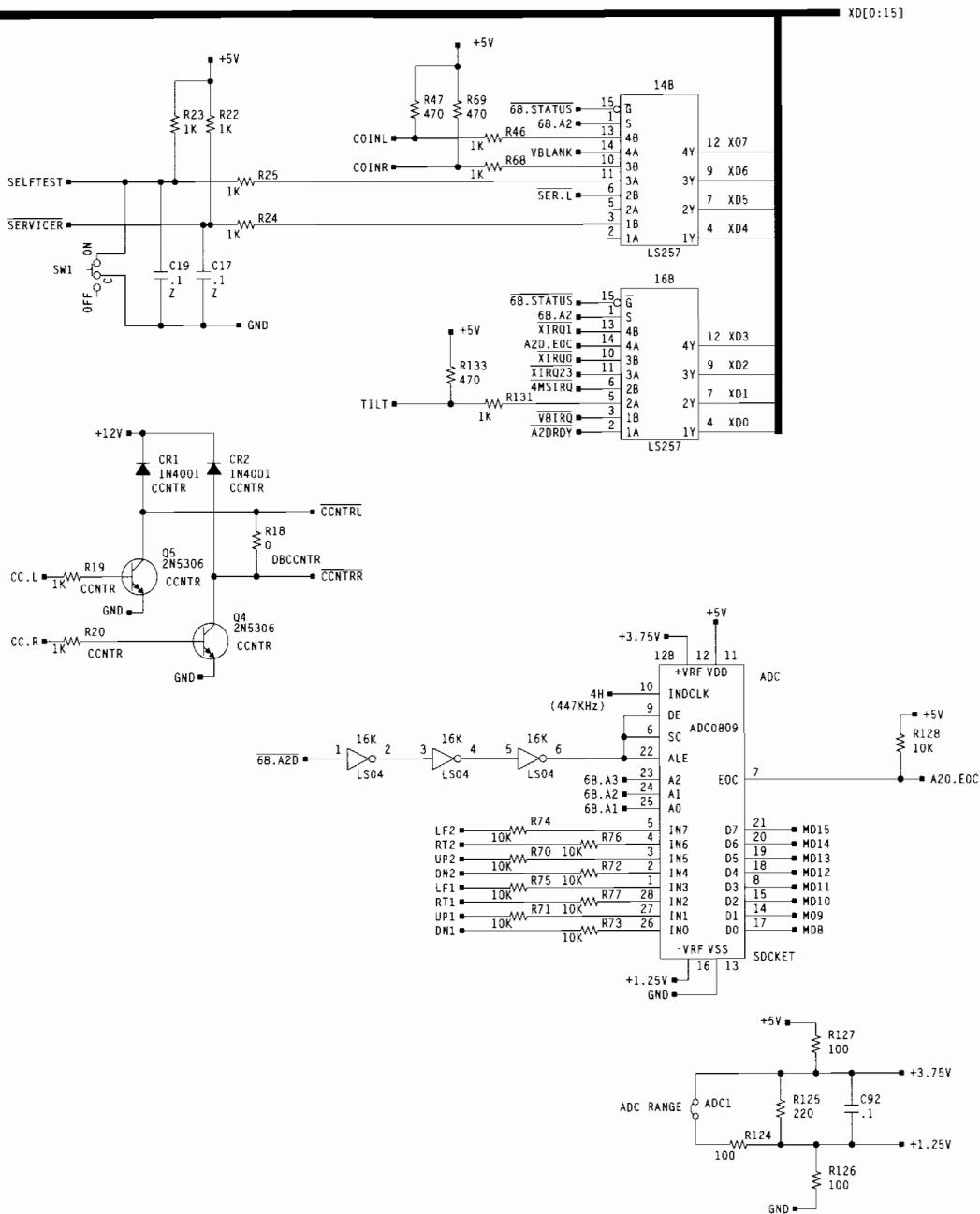
Figure 5-1 Primal Rage Game (GT) PCB Schematic Diagram, Continued
