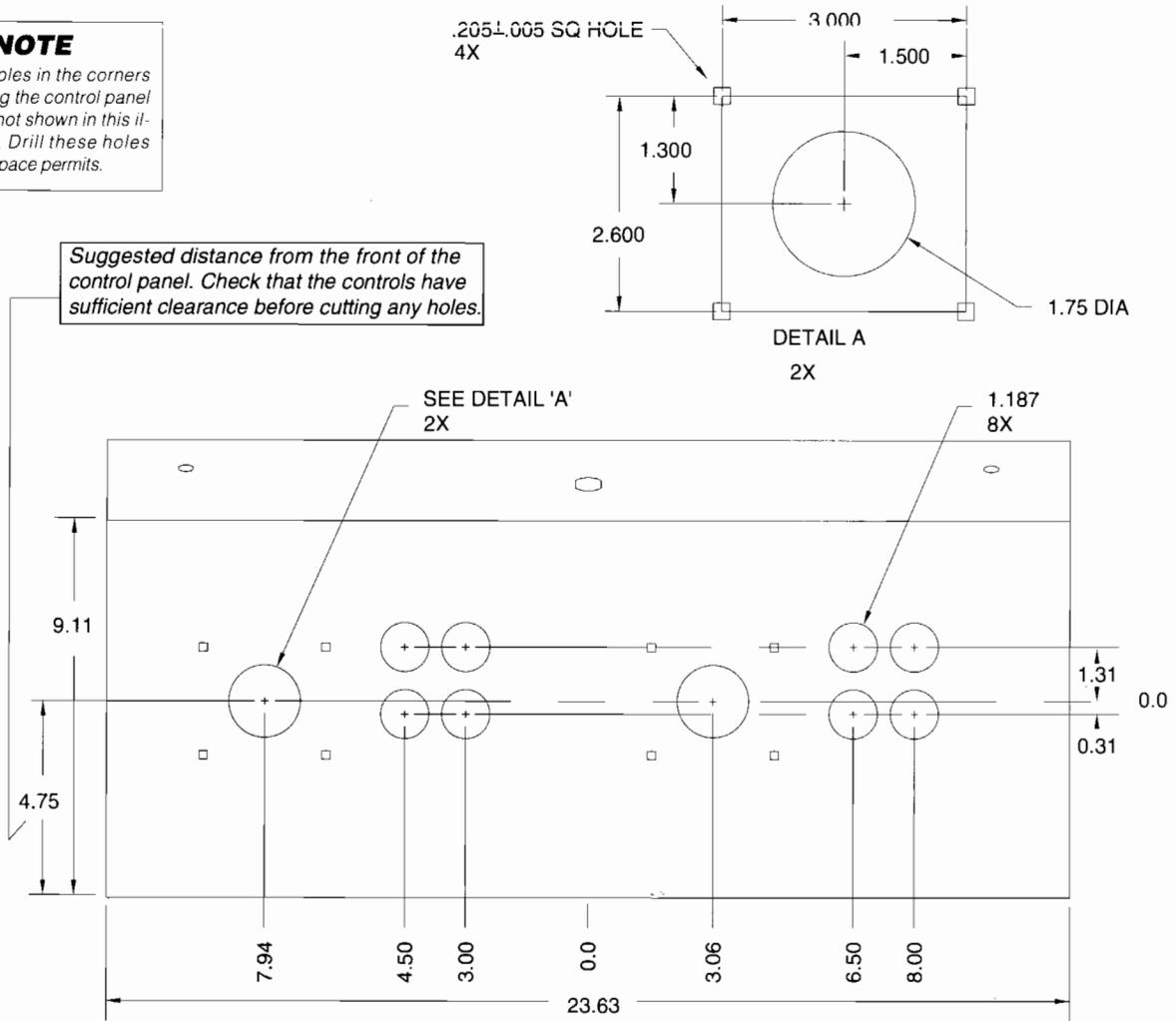
**Figure 1-1 Locations of Control Panel Holes to be Drilled**
