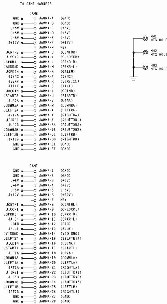
**Figure 5-3 JAMMA Filter PCB Schematic Diagram**
