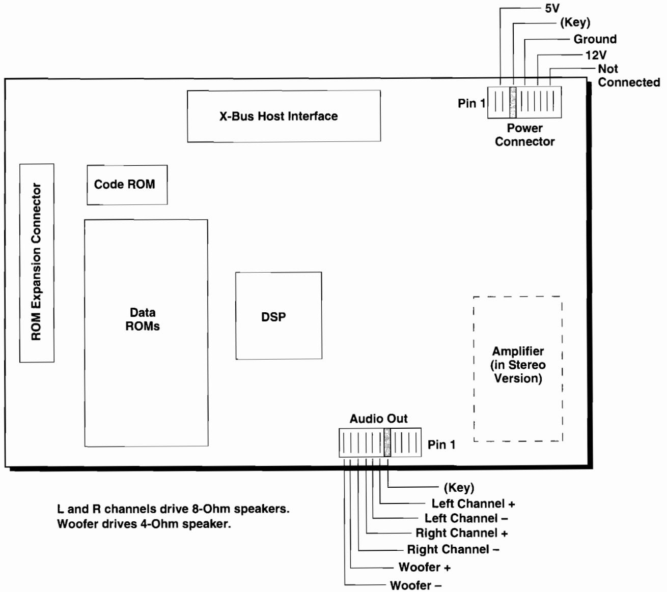
**Figure 5-4 CH31\_2 (CAGE Audio) Board Block Diagram**
