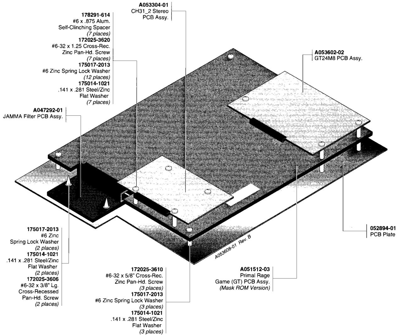
**Figure 4-2 Board Stack Assembly**
