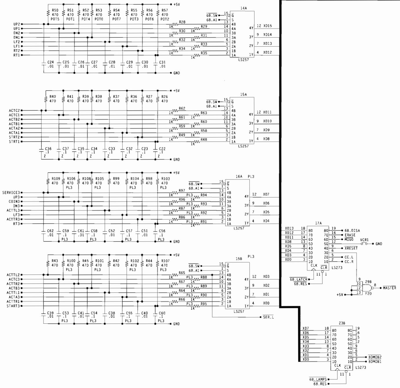
Figure 5-1 Primal Rage Game (GT) PCB Schematic Diagram
