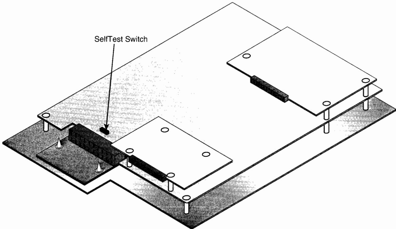
**Figure 2-1** Location of Self-Test Switch
