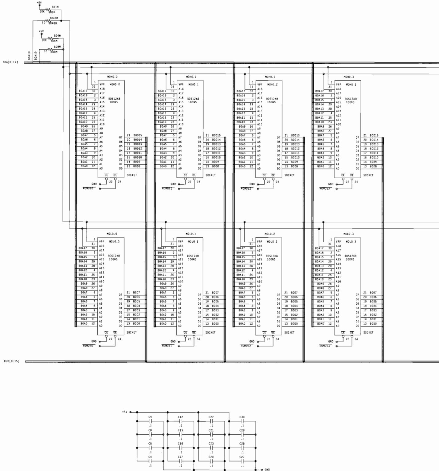
**Figure 5-2 GT24M8 PCB Schematic Diagram**
