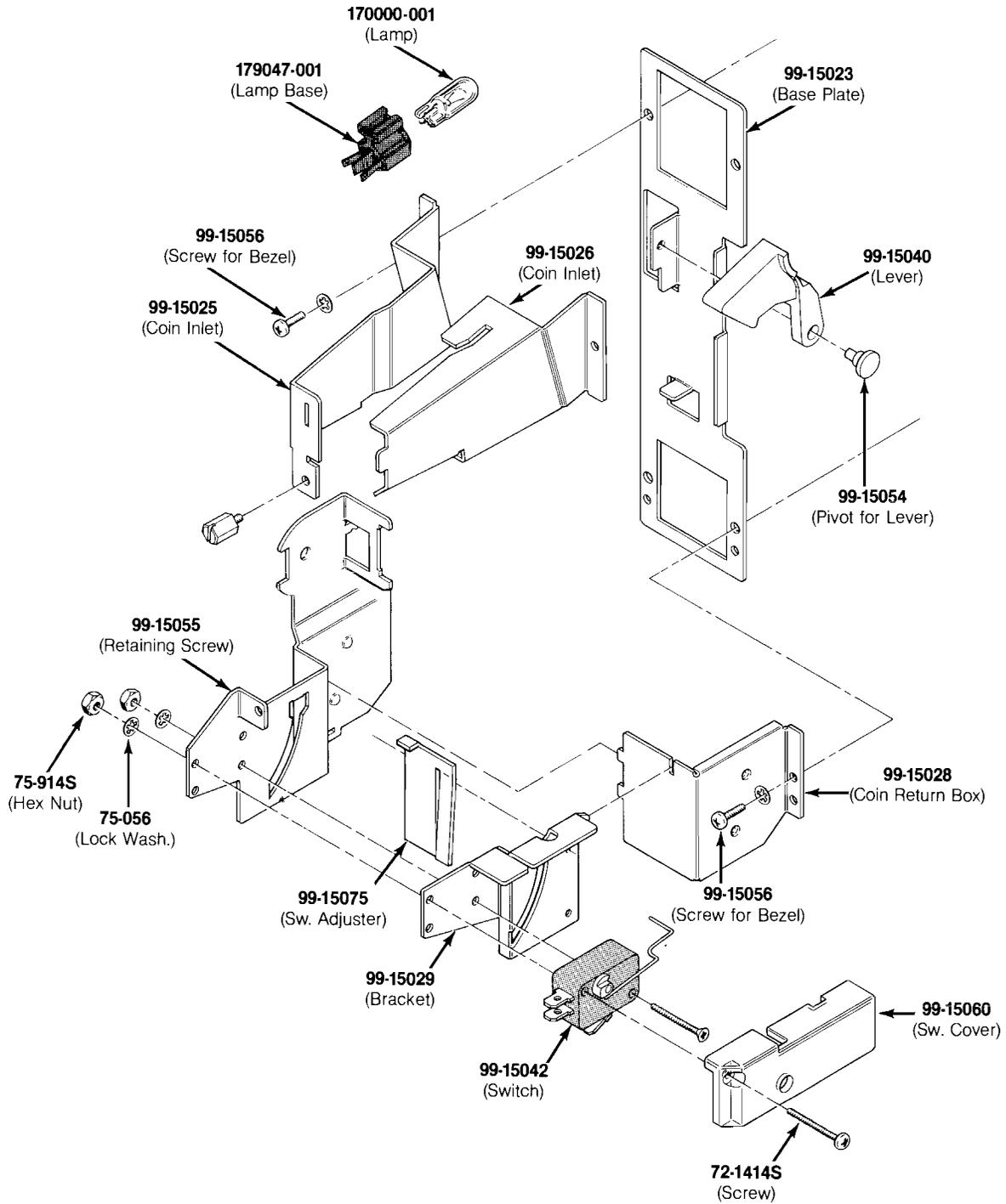
**Figure 3-16 Vertically Mounted Coin Door
