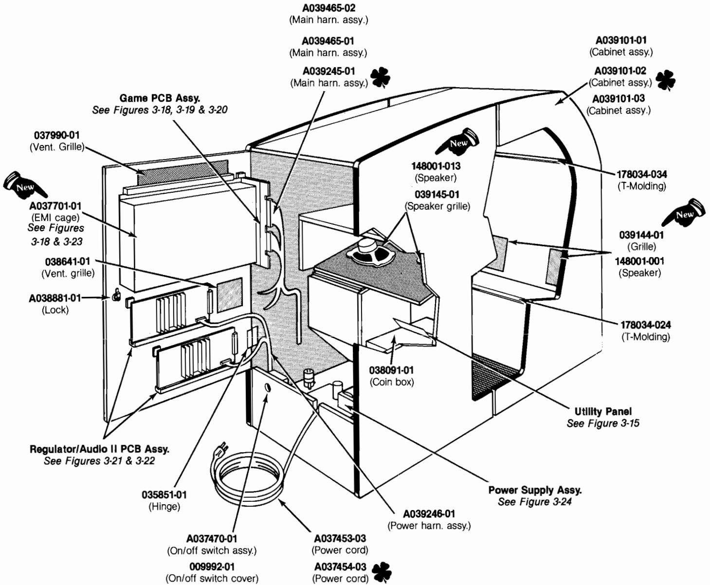
**Figure 3-2 Cabinet-Mounted Assemblies**
