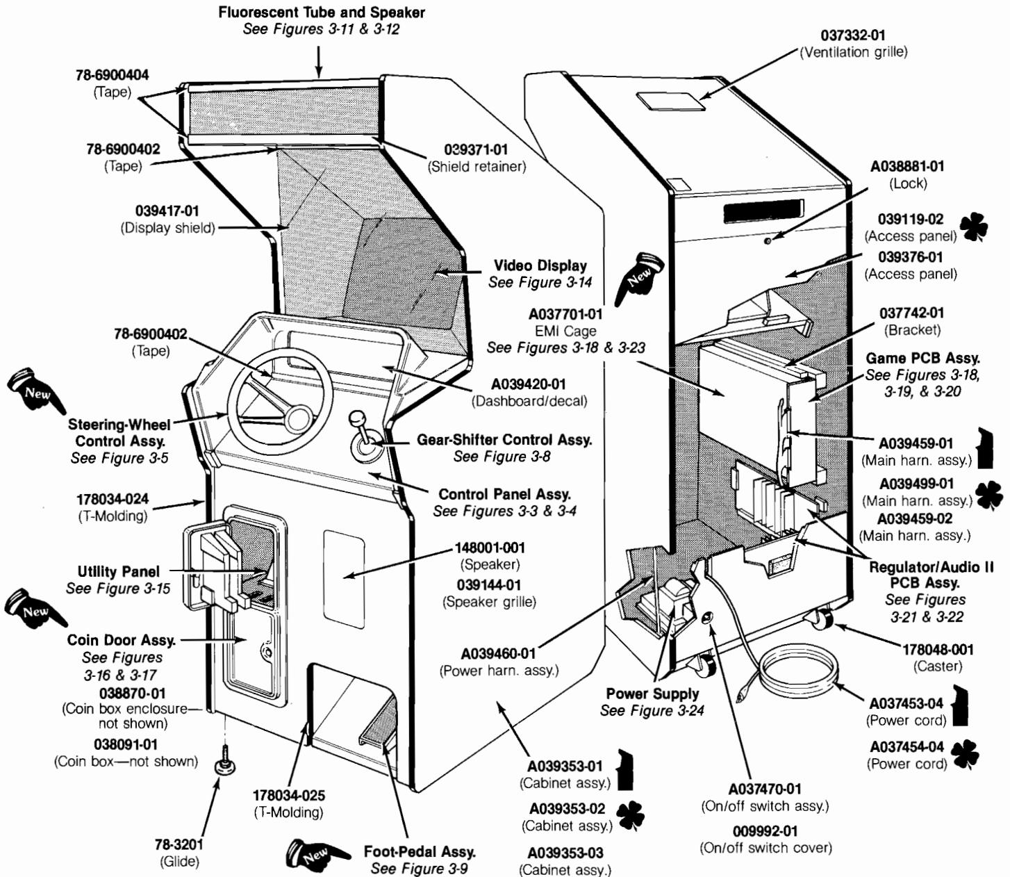
**Figure 3-1 Cabinet-Mounted Assemblies**
