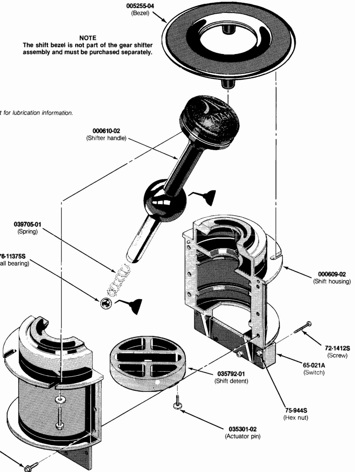
**Figure 3-8 Gear-Shifter Control Assembly
