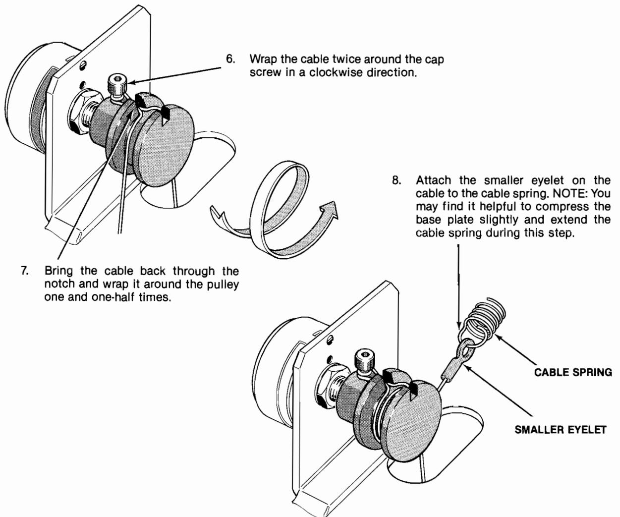
**Figure 3-10 Foot-Pedal Pulley Cable Rewinding, continued**
