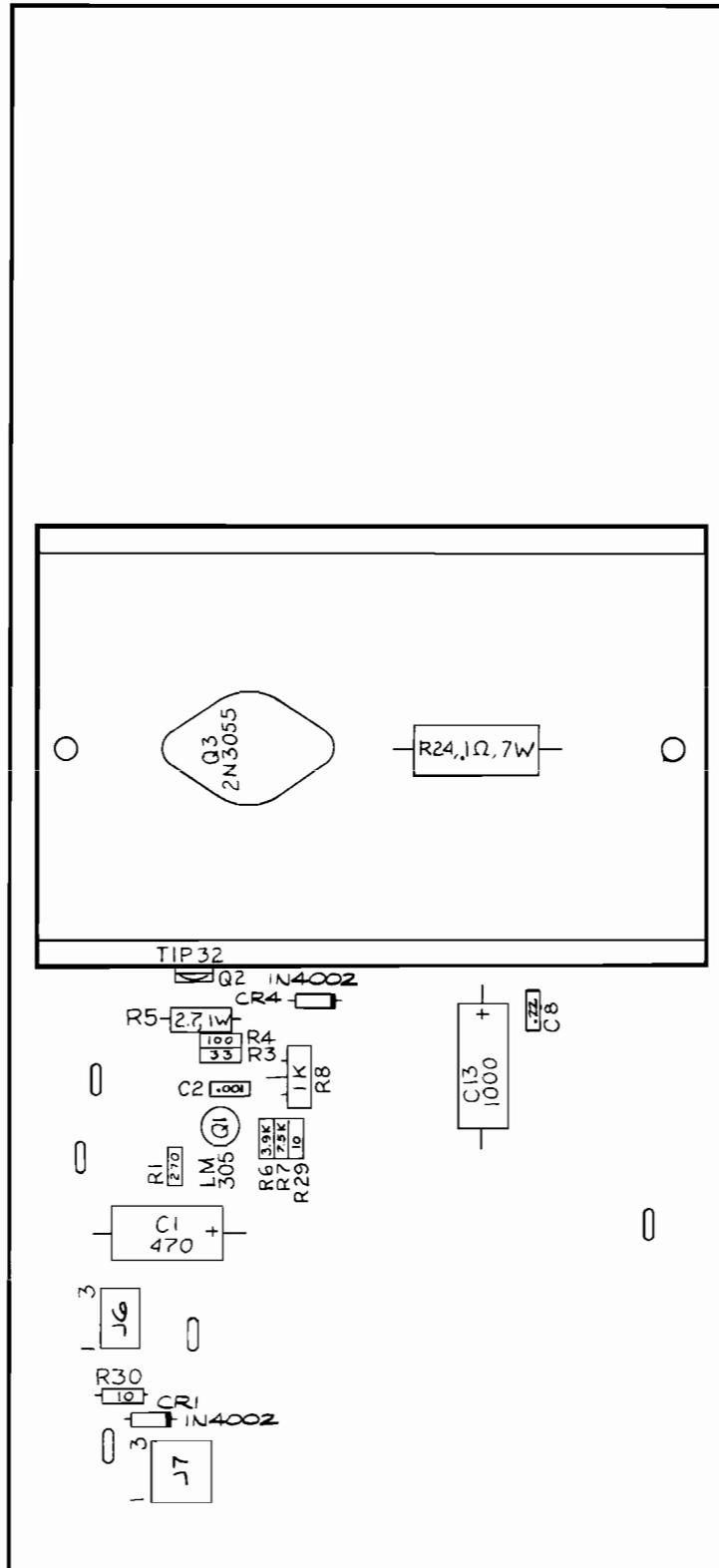
**Figure 3-22 Regulator/Audio II PCB Assembly**
