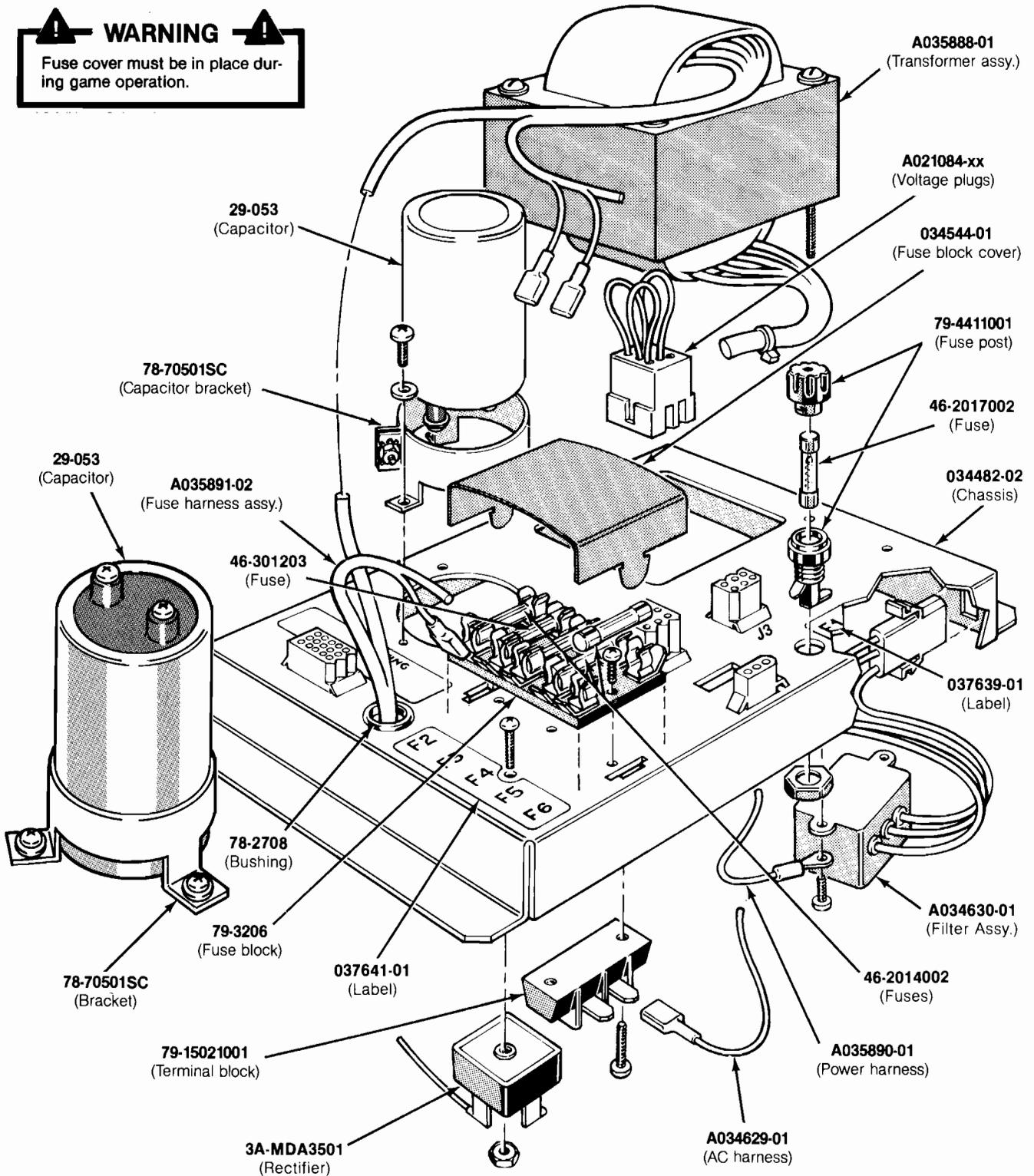
Figure 3-24 Power Supply Assembly
