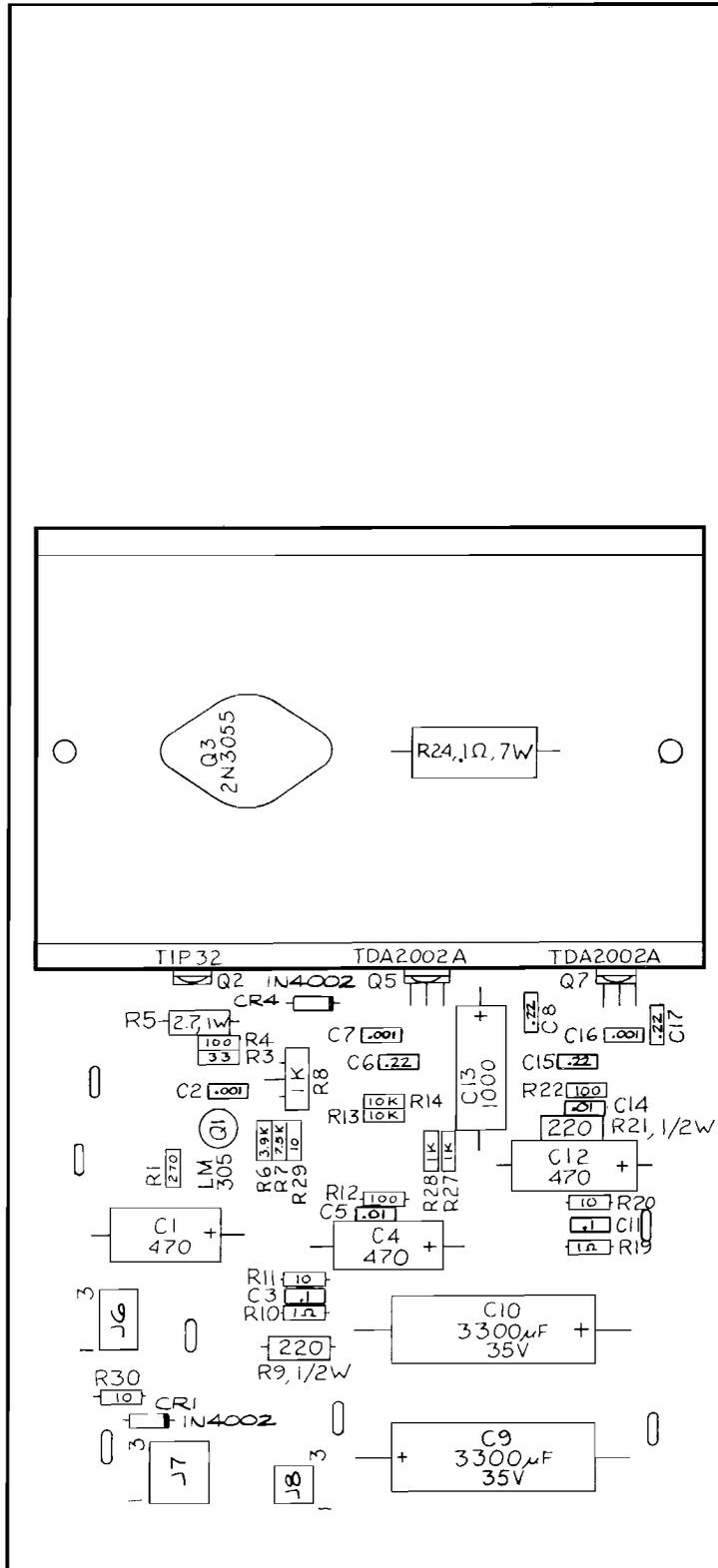
Figure 3-21 Regulator/Audio II PCB Assembly
