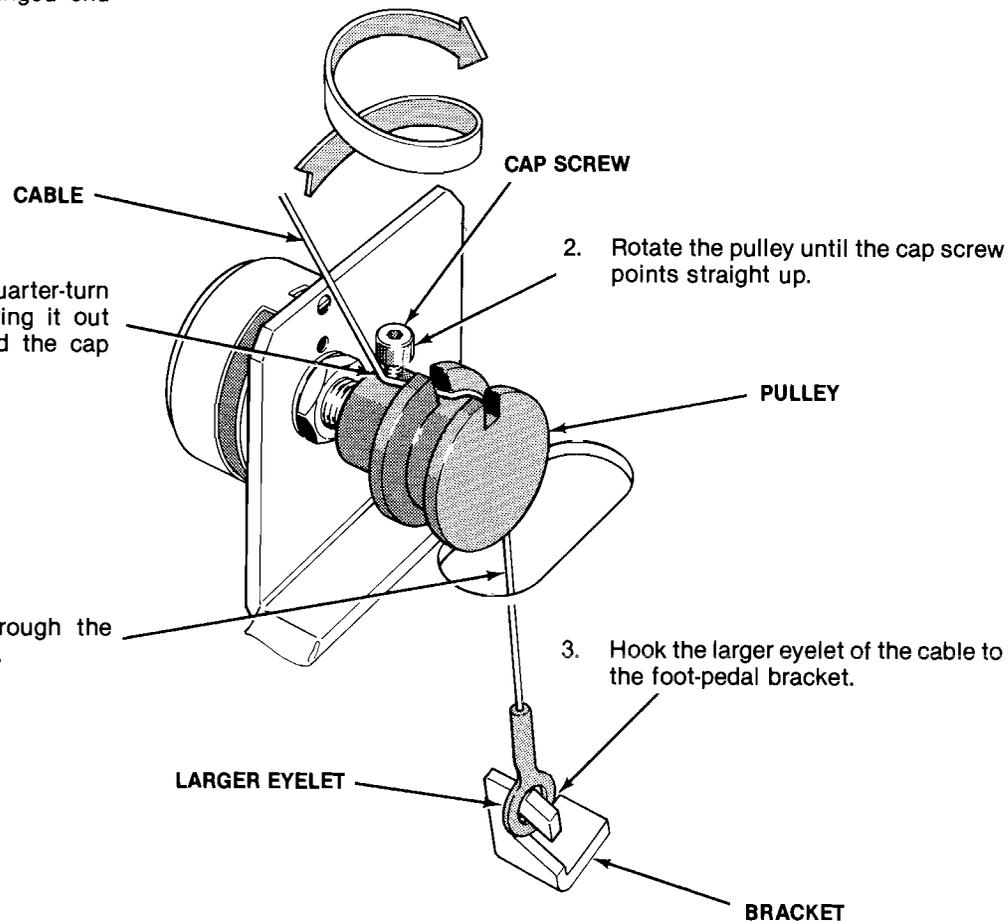
**Figure 3-10 Foot-Pedal Pulley Cable Rewinding**
