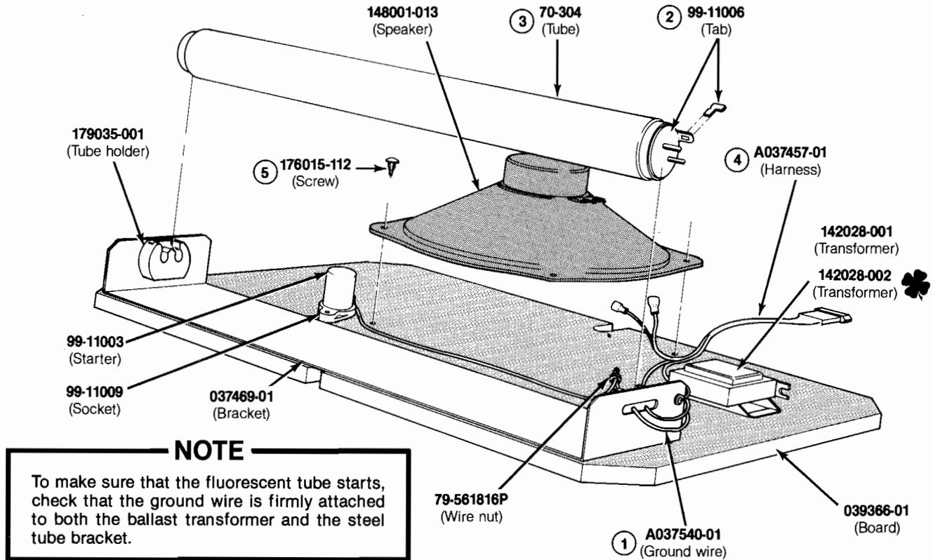
**Figure 3-12 Fluorescent Tube and Speaker Board Assembly**
