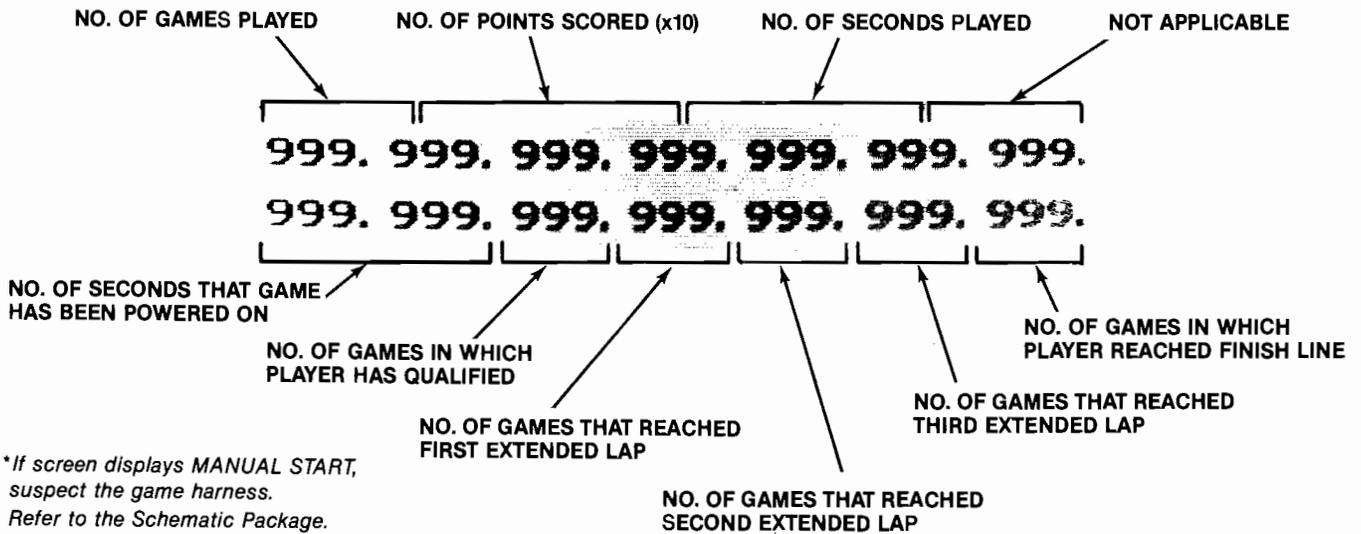
*\*If screen displays MANUAL START, suspect the game harness. Refer to the Schematic Package.*
