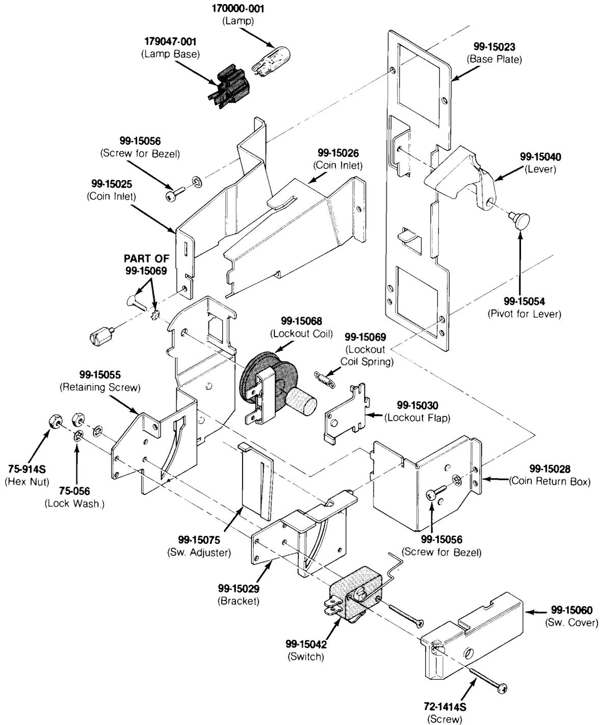
**Figure 3-13 Vertically Mounted Coin Door
