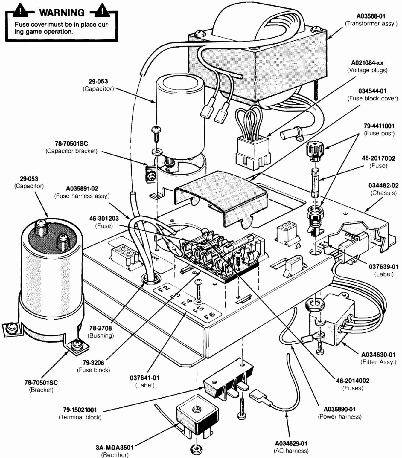
Figure 3-21 Power Supply Assembly
