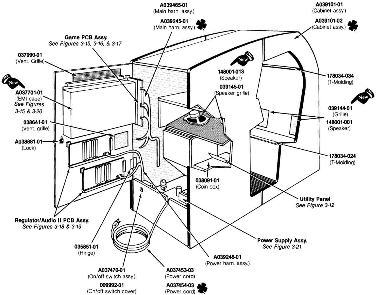
**Figure 3-2 Cabinet-Mounted Assemblies**
