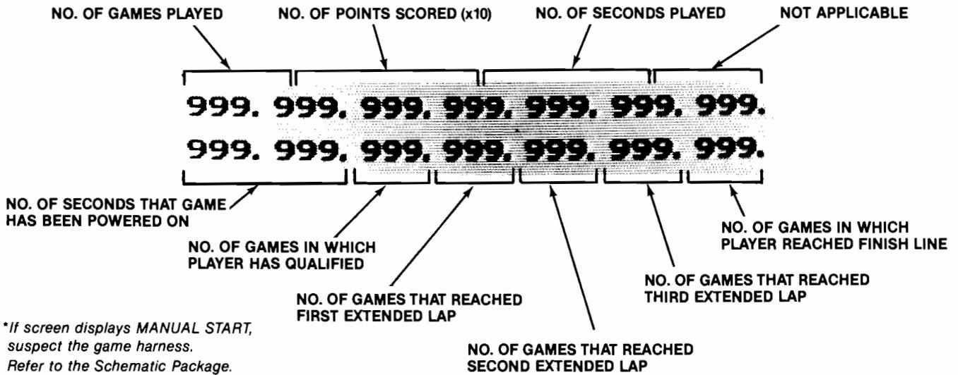
Figure 1-5 Self-Test Display
