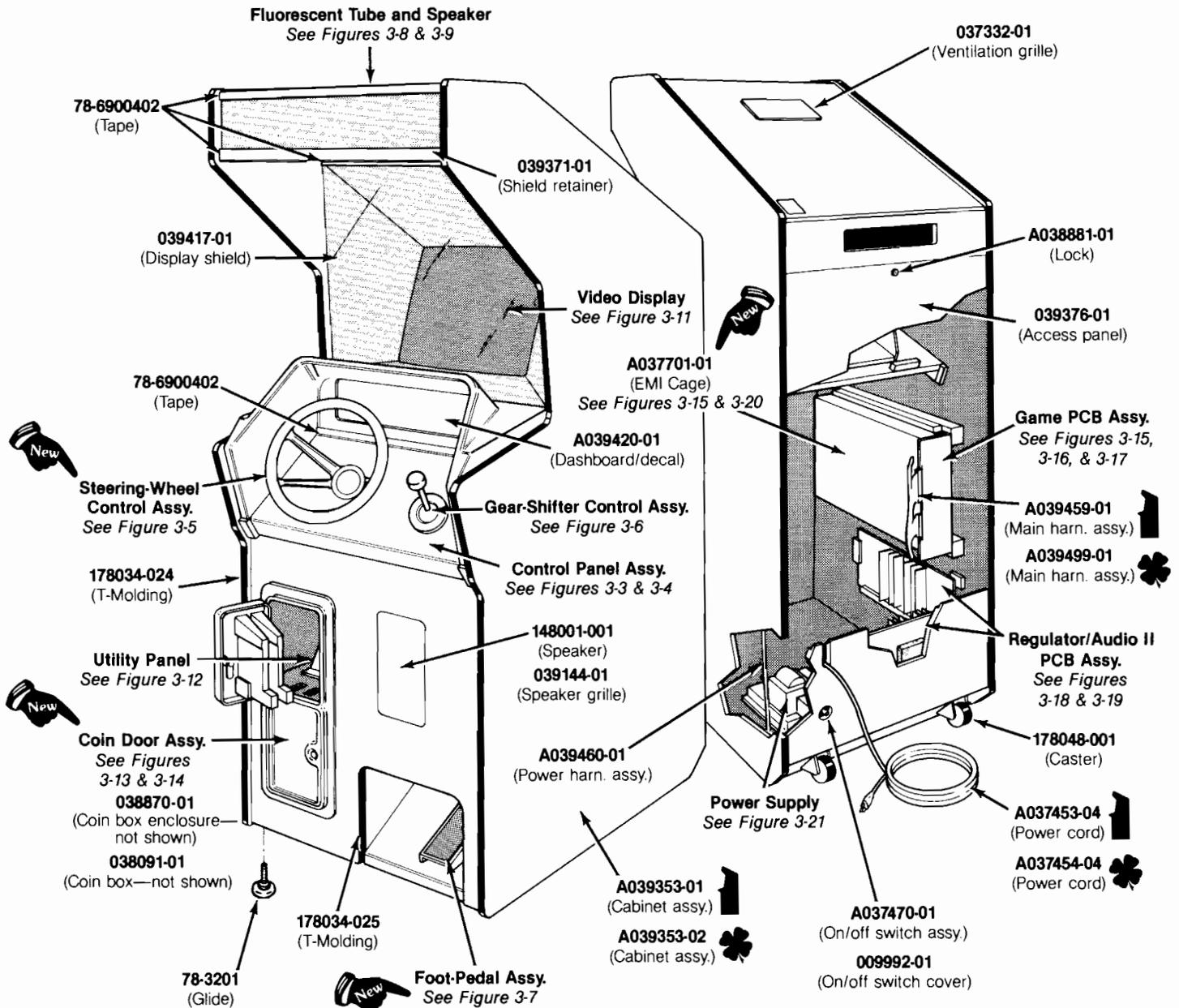
**Figure 3-1 Cabinet-Mounted Assemblies**
