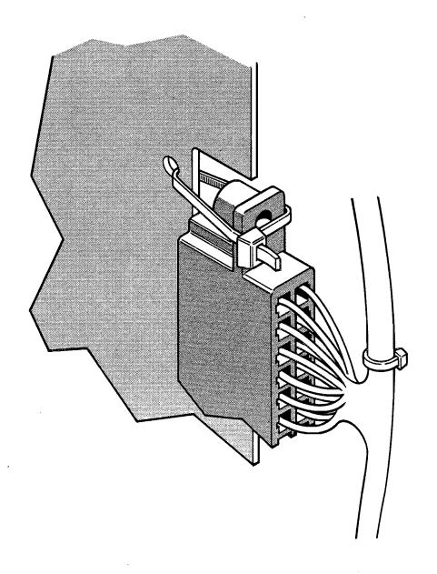
Figure 5 PCB Edge-Connector Wire-Tie Installation
