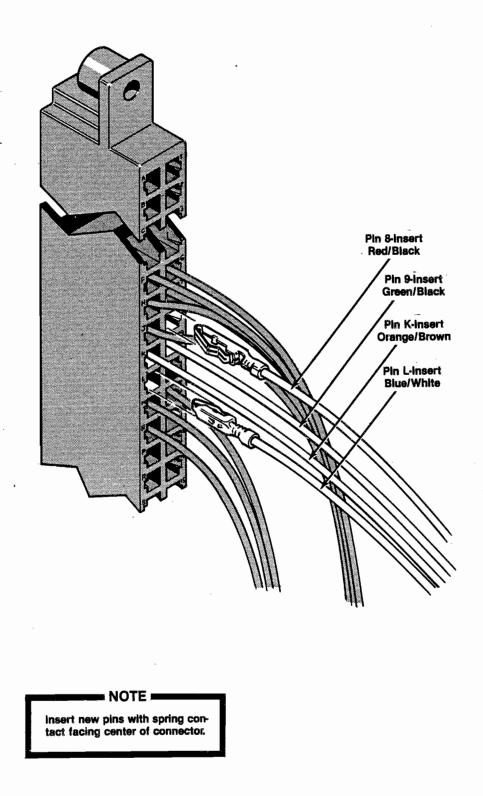
Figure 4 Harness Wire Installation
