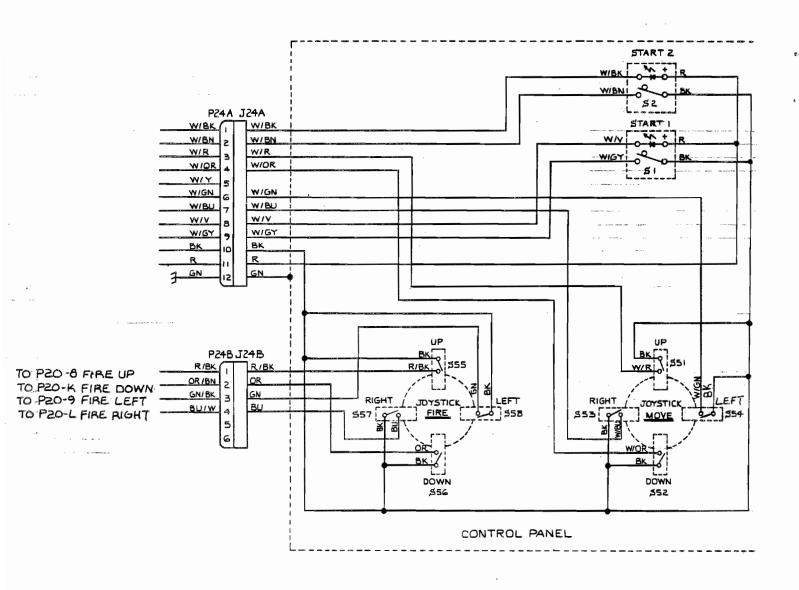
Figure 6 Sheet 1B (Gravitar Main Wiring Diagram) Changes
