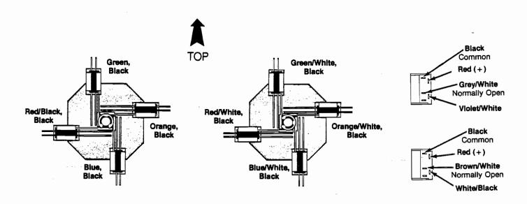
Figure 3 Assembling the Control Panel
