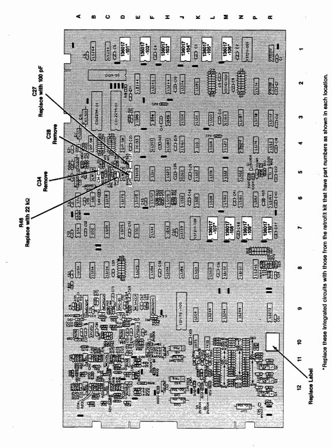
Figure 2 Location of PCB Components Affected by Retrofit
