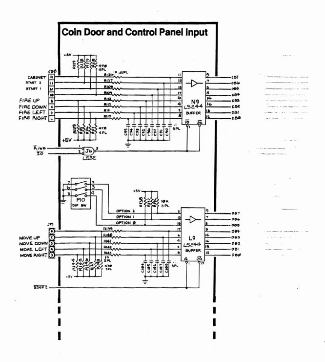
Figure 7A Sheet 5A (Gravitar PCB Schematic Diagram) Changes
