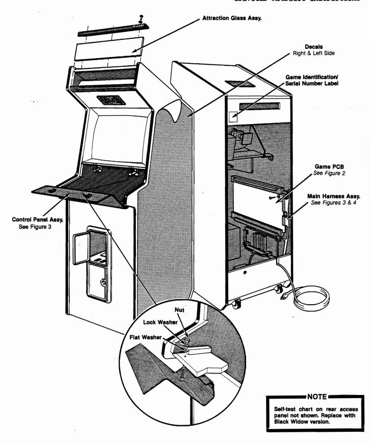
Figure 1 Location of Gravitar Parts Affected by Retrofit
