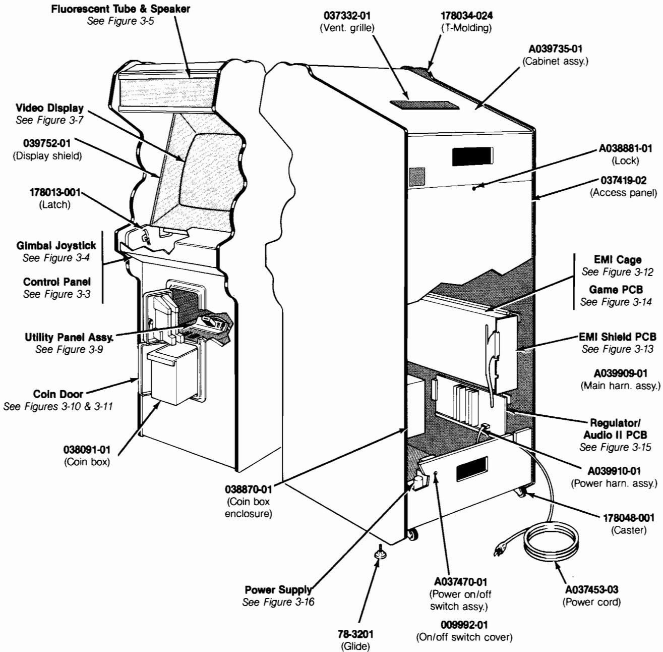
**Figure 3-1 Cabinet-Mounted Assemblies
