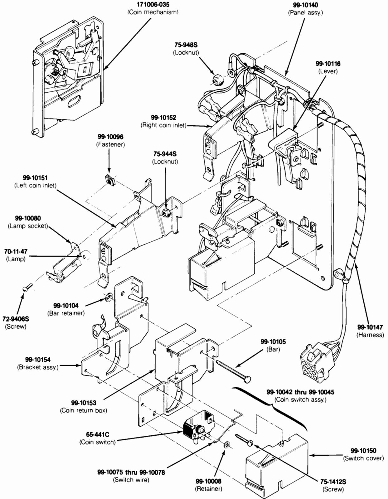
**Figure 3-11 American-Made Coin Door Assembly
