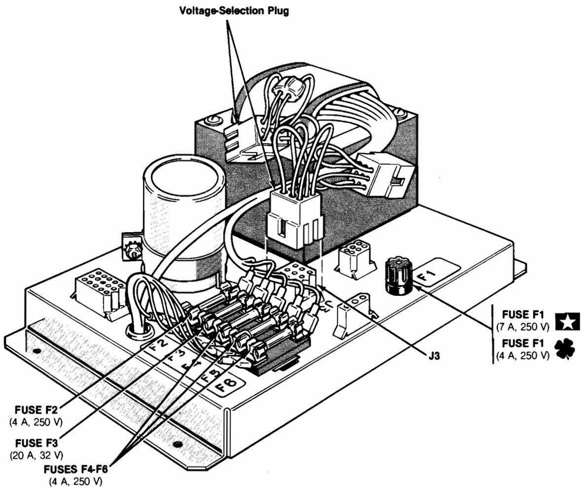
**Figure 1-3 Voltage-Selection Plug and Fuses**
