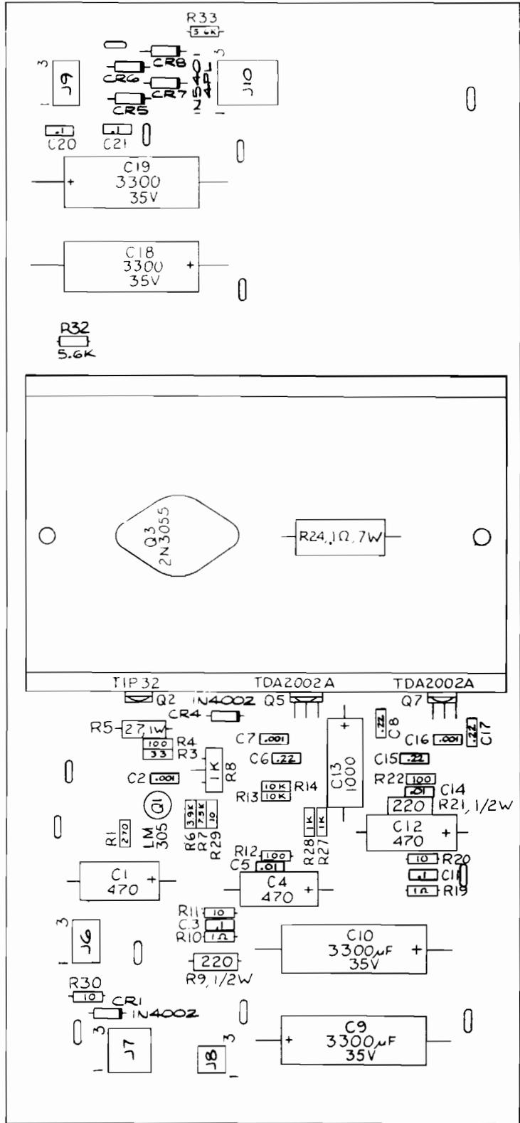
**Figure 3-15 Regulator/Audio II PCB Assembly**
