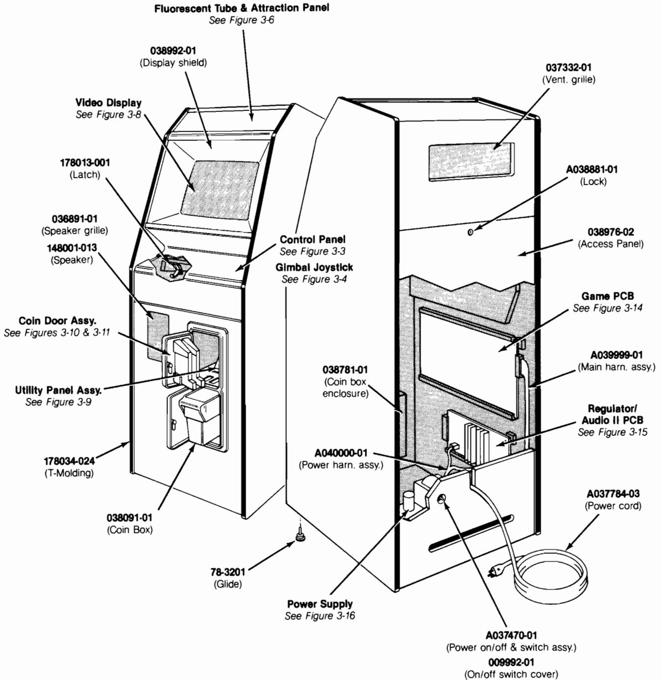
**Figure 3-2 Cabinet-Mounted Assemblies**
