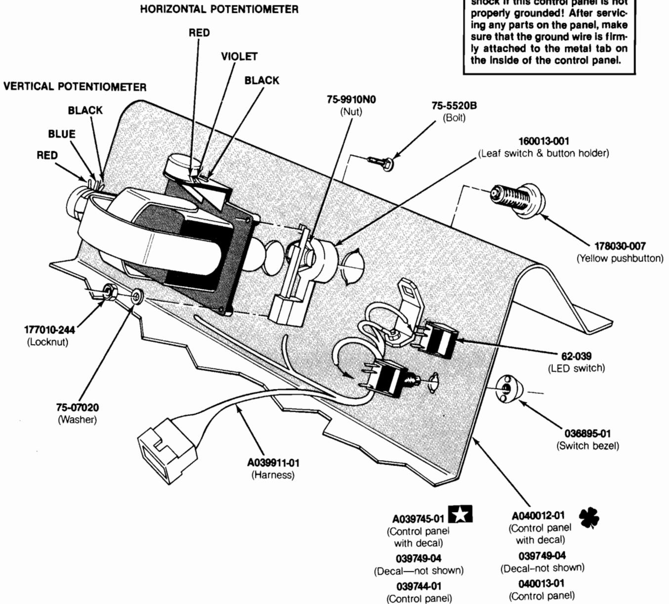
**Figure 3-3 Control Panel Assembly**
