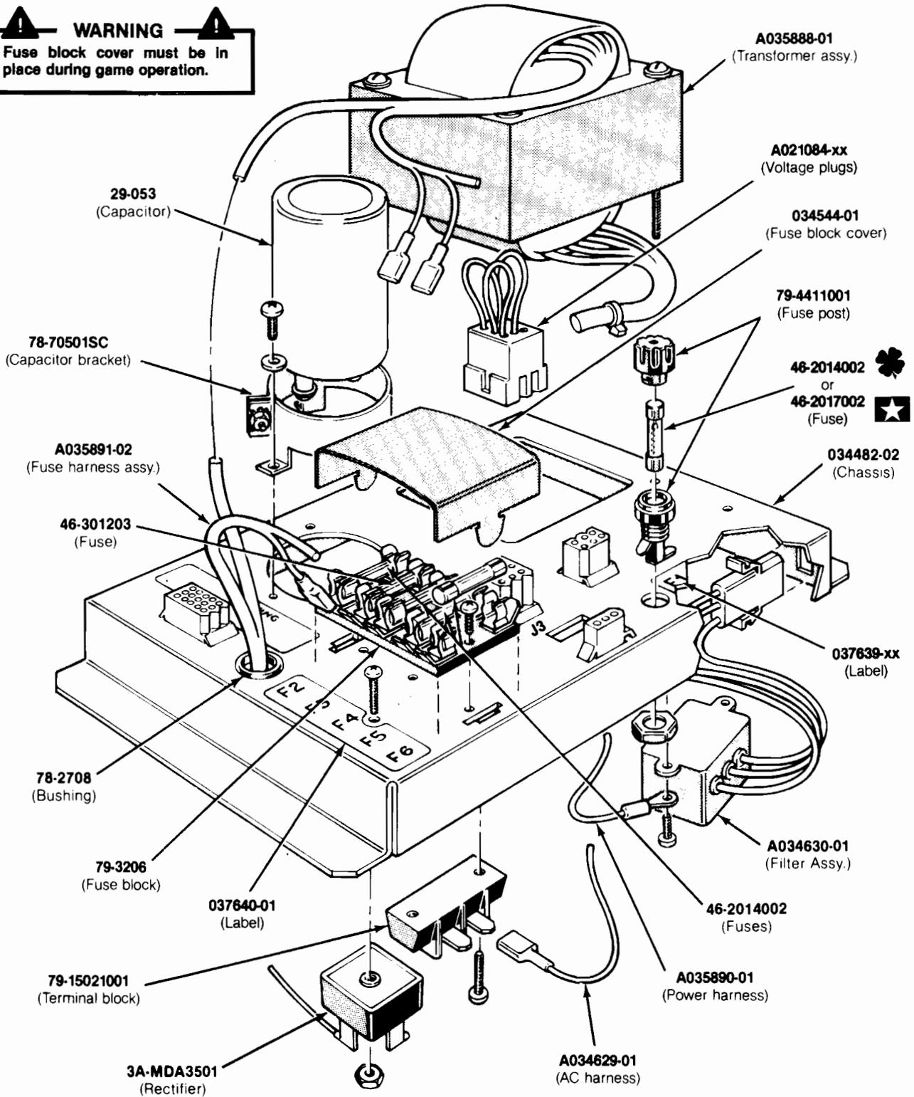
**Figure 3-16 Color Raster-Scan Power Supply Assembly
