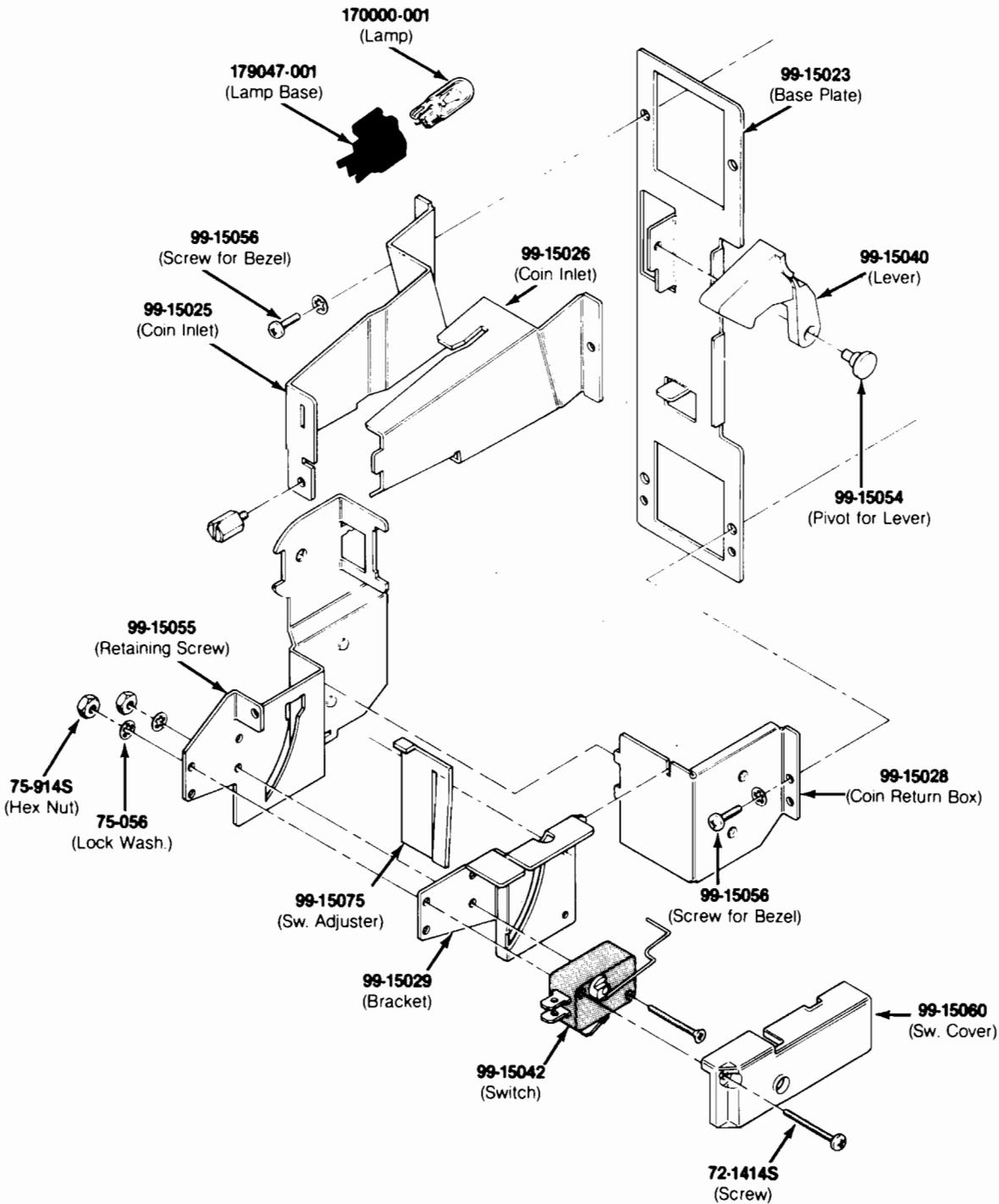
**Figure 3-10 Vertically Mounted Coin Door
