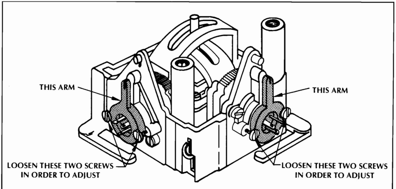
Figure 5-4 Detail View of Joystick Assembly
