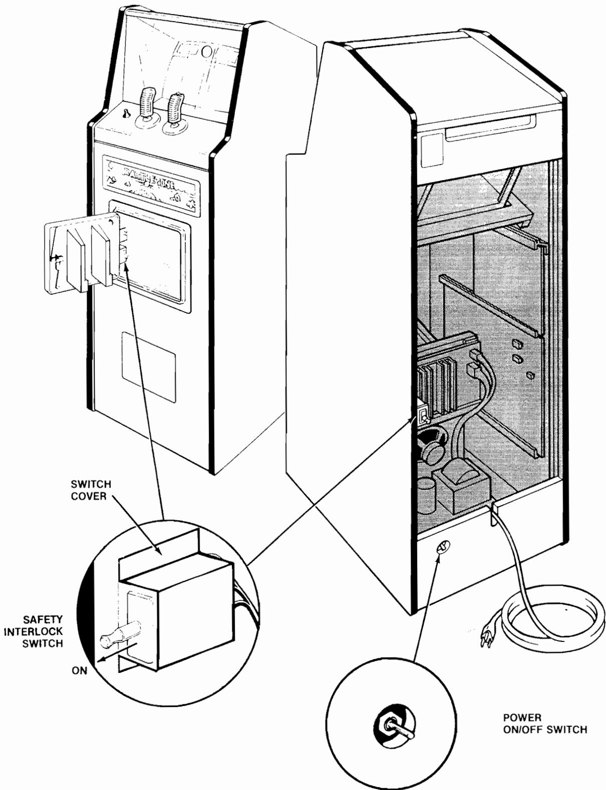
Figure 4 Interlock and Power On/Off Switches
