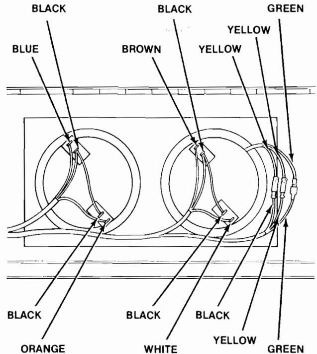
Repairs on the control handle would probably only involve replacement of switches. When removing a switch, be careful not to lose the small clear plastic actuator pins that sit above the white switch actuators. Note: the flat head of the pin must **always** face towards the switch actuator.
