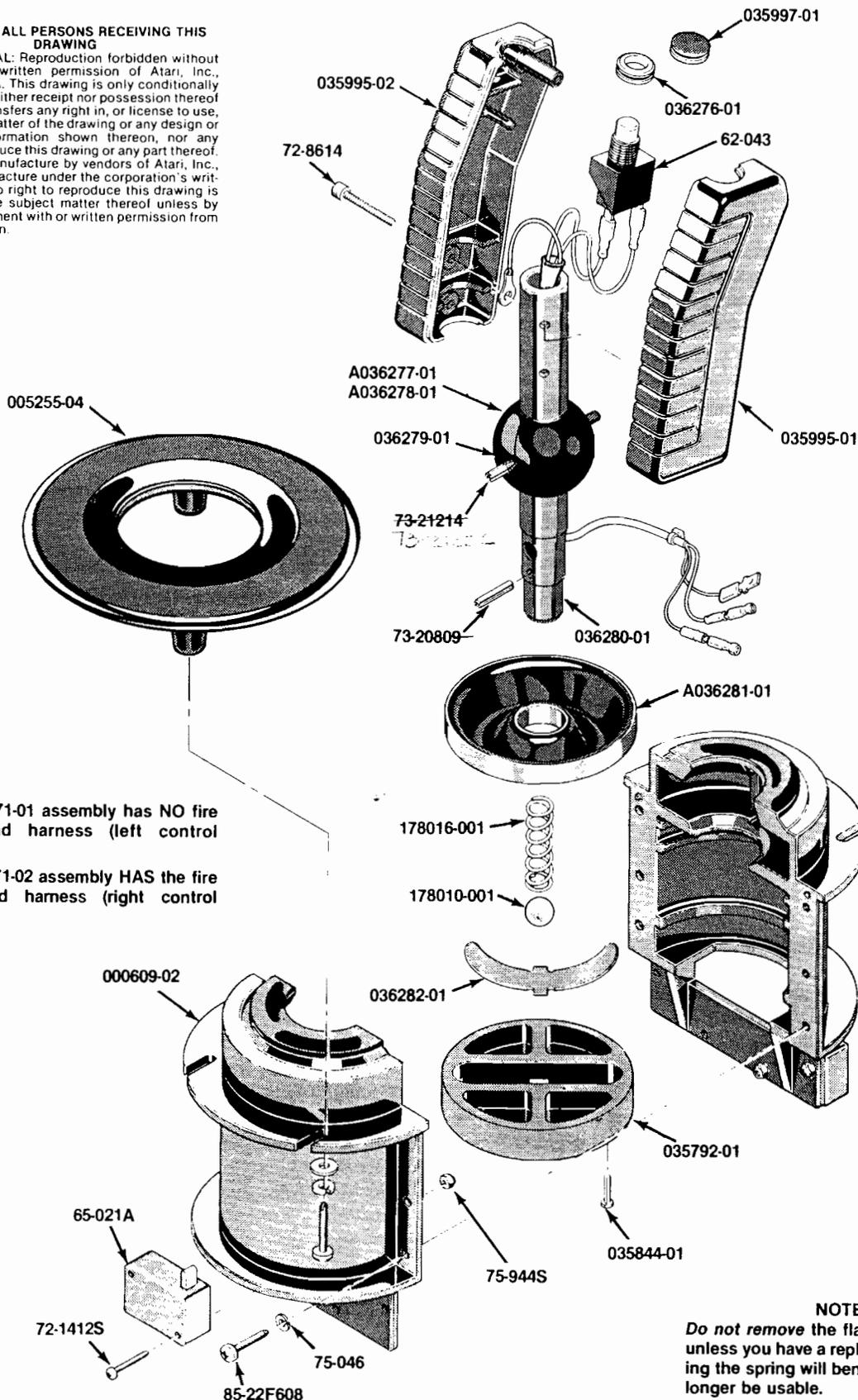
The A036271-01 assembly has NO fire switch and harness (left control handle).
