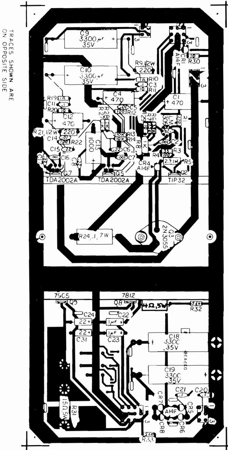
Figure 24 Regulator/Audio II PCB Assembly
