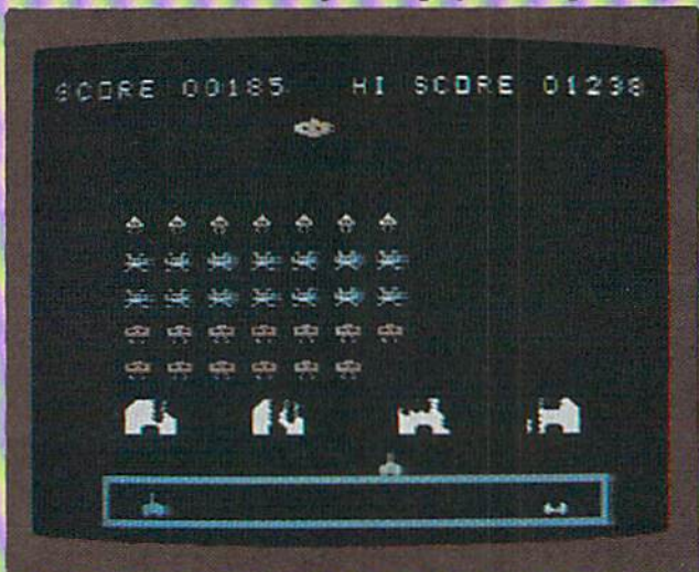
The TI-99/4A is capable of simultaneously manipulating 32 sprites. This adds more detail to Space Invaders graphics than the Vic-20 version can offer.
