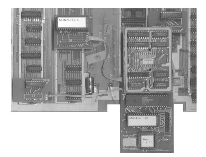
Double check that all the MultiPac boards are fully plugged in, and that there are no pins bent out or missing the sockets.
