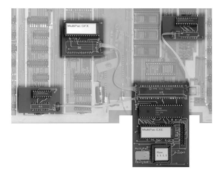
Once all the MultiPac boards are installed, replace the "Z-80 Sync Bus Controller" board at location 6D. The chips on the "Z-80 Sync Bus Controller" board should all have their notches facing the same direction as the chips on the game Board. The chips on the MultiPac boards should also be facing the same direction as the chips on the game board. Be careful to keep the wire going to "7F" away from the socket at 6D.
