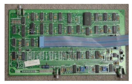
Solder the jumper wire from Pin1 of the 74LS244 at location E2, to pin 19 on the DIP20 socket at location G3 We chose to make these connections neatly on the underside of the board.
