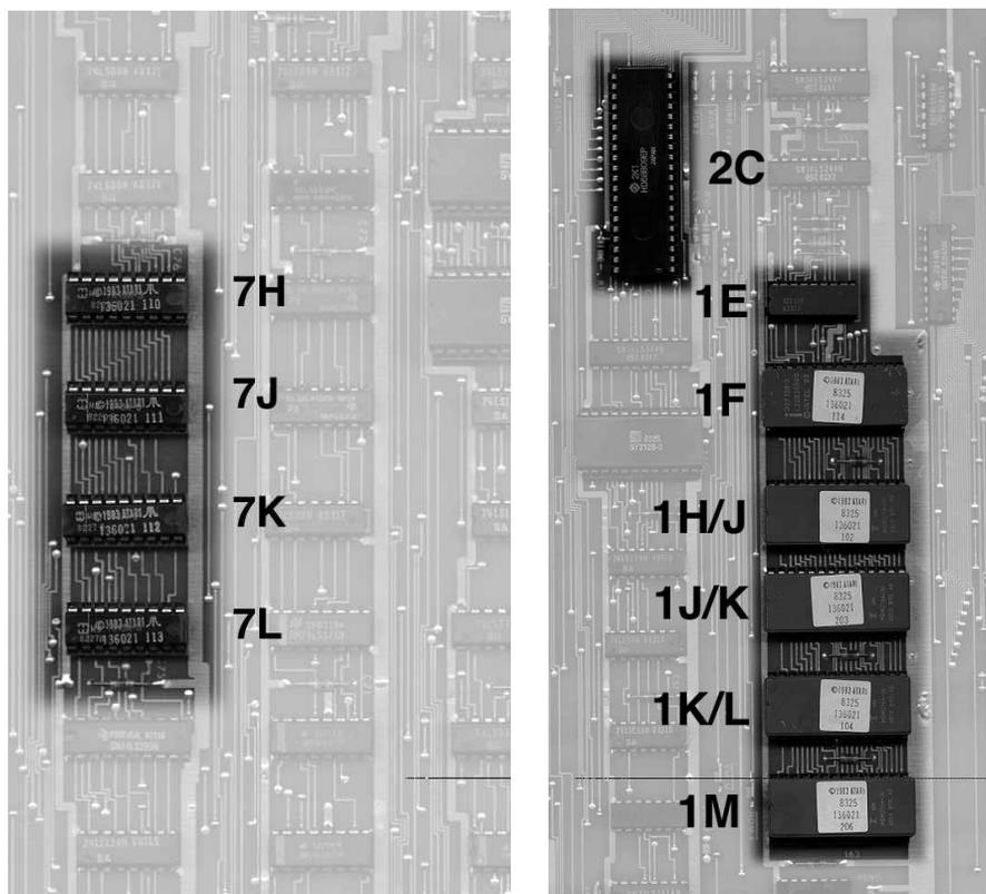
You’ll be replacing the PROMs (on the left, 7H-7L); replacing the EPROMs (on the right, 1F-1M); removing the NOVRAM at 1E; as well as soldering on a wire to the 6809 in location 2C and placing the daughtercard in the socket at 1H/J and 1E.
