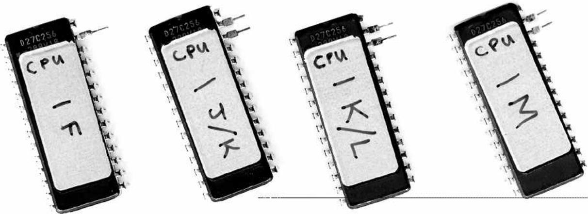
Now locate your "SND" EPROMs and the "AVG" EPROM. This will be the same drill as before, bend the correct pins out, but not straight out...
