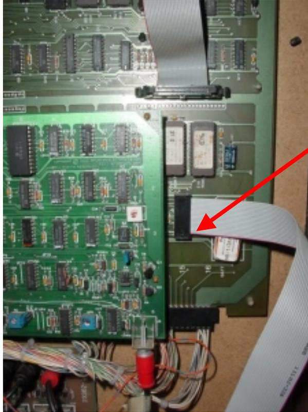
**Pin 1 and cable stripe is here. Your cable may be crimped on the other side, use the Pin 1 and stripe location as the guide**
