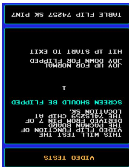
*The Video Flip Test in Flipped Mode*
